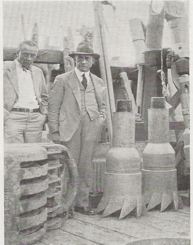
Arthur Beeby Thompson, noted English geologist, right, and F. W. Lake, general superintendent at Santa Fe Springs, looking over the new hole straightening tool recently invented by F. F. Hill, manager of field operations.
