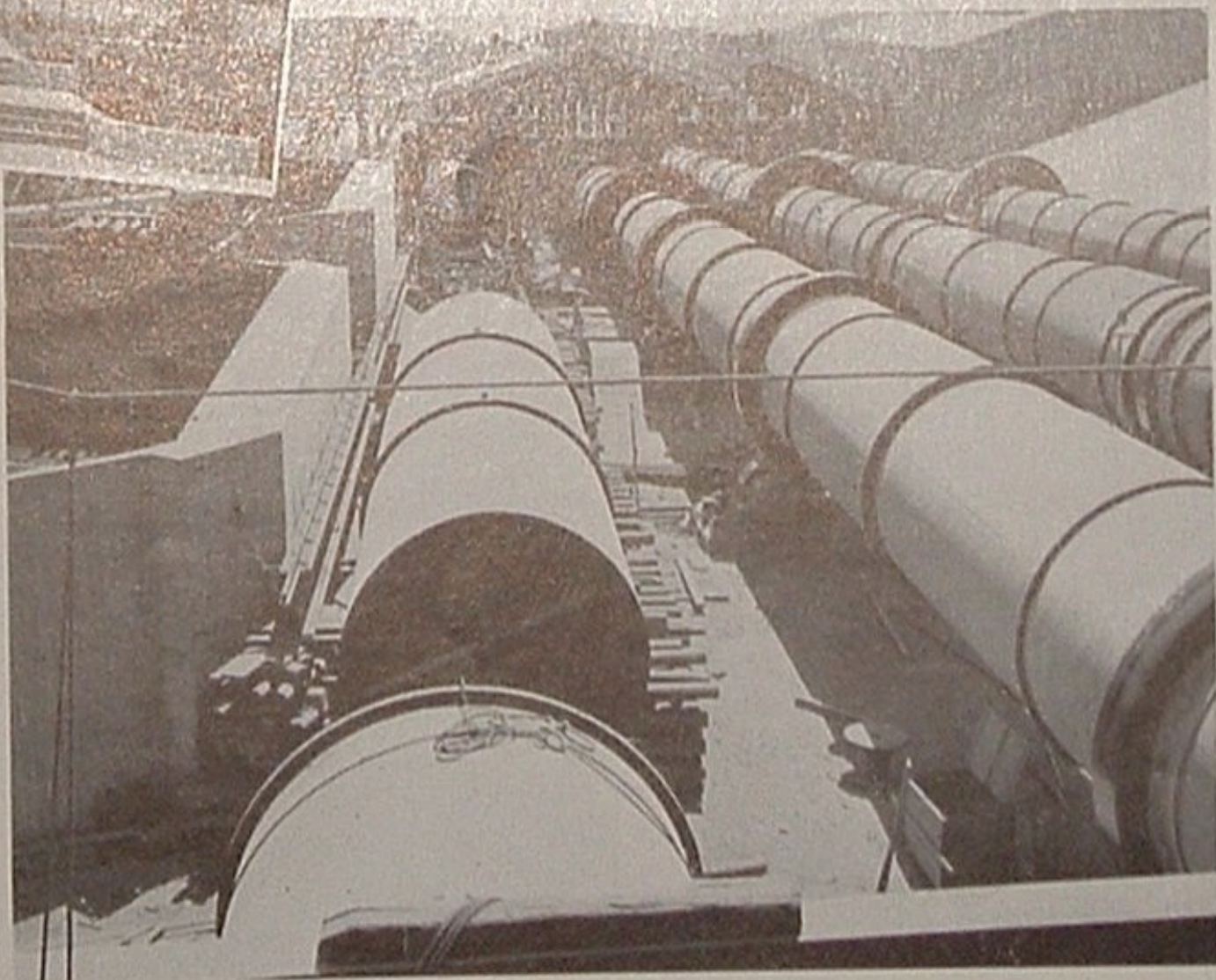
Right: In these large rotary kilns, magnesium oxide is formed. Ore for the kilns comes from large deposits near Luning, Nevada.
