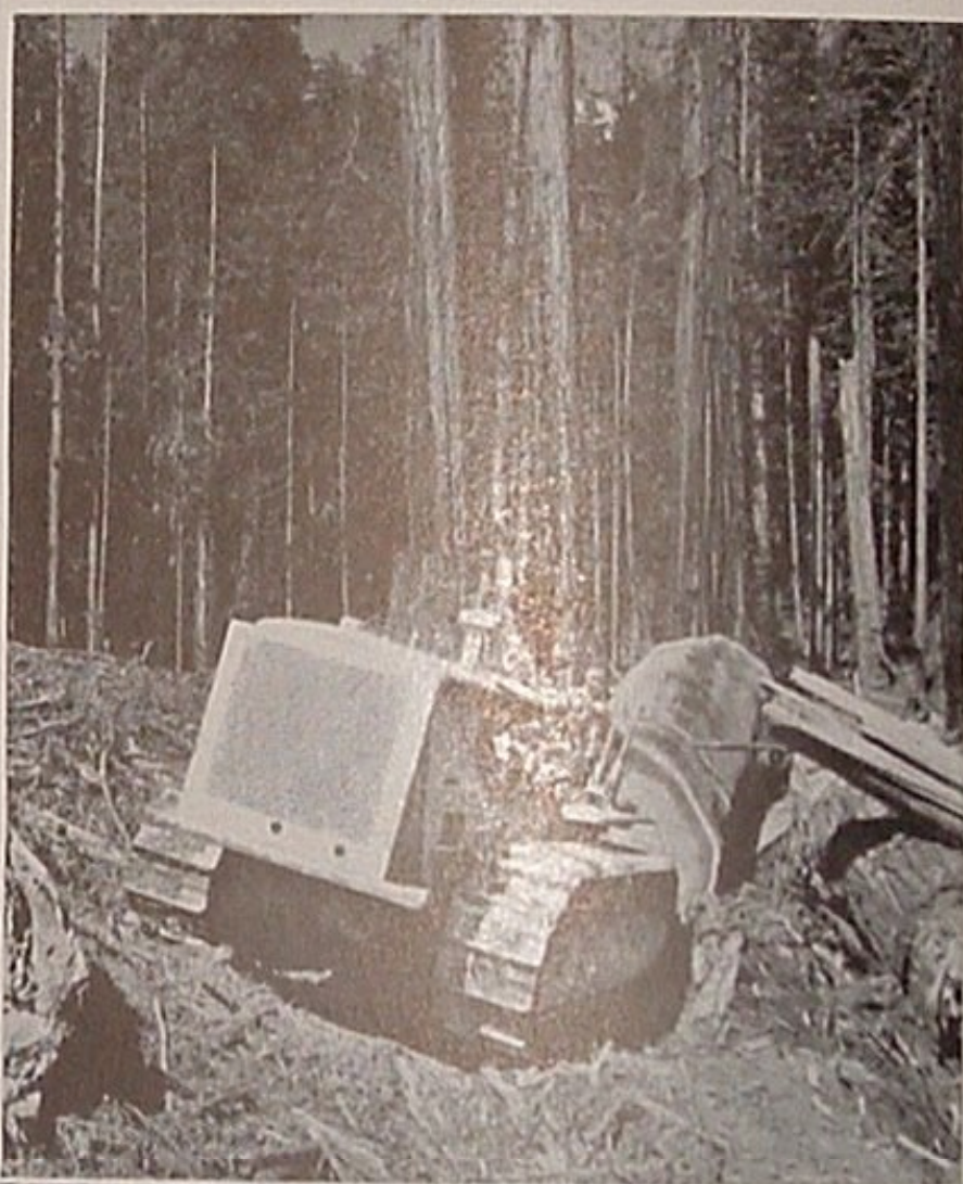
The lumber industry makes good use of Caterpillars. The RD8 Diesel above is skidding redwood logs near Cranell, California.
