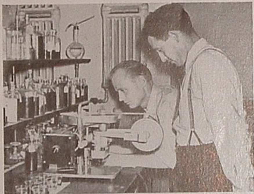
Above: C. Jones and M. T. Flaxman use the Faville-LeValley tester to determine the film strength of various lubricating oils.
