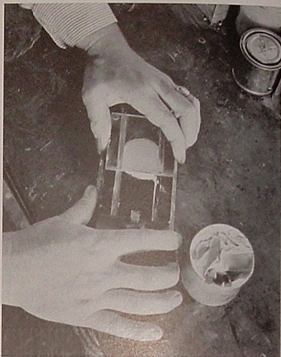
The covering quality of paints is measured by the "Cryptometer" seen above in operation.
