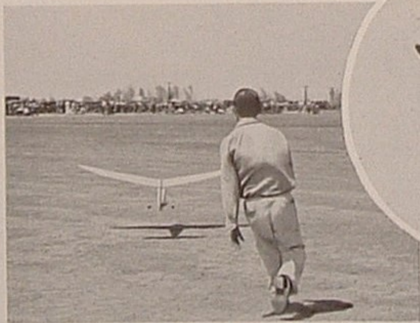
The model planes are very powerful for their size and take off at a terrific clip. Once off the ground they fly gracefully until the timer shuts the motor off, then they nose down and glide toward earth.
