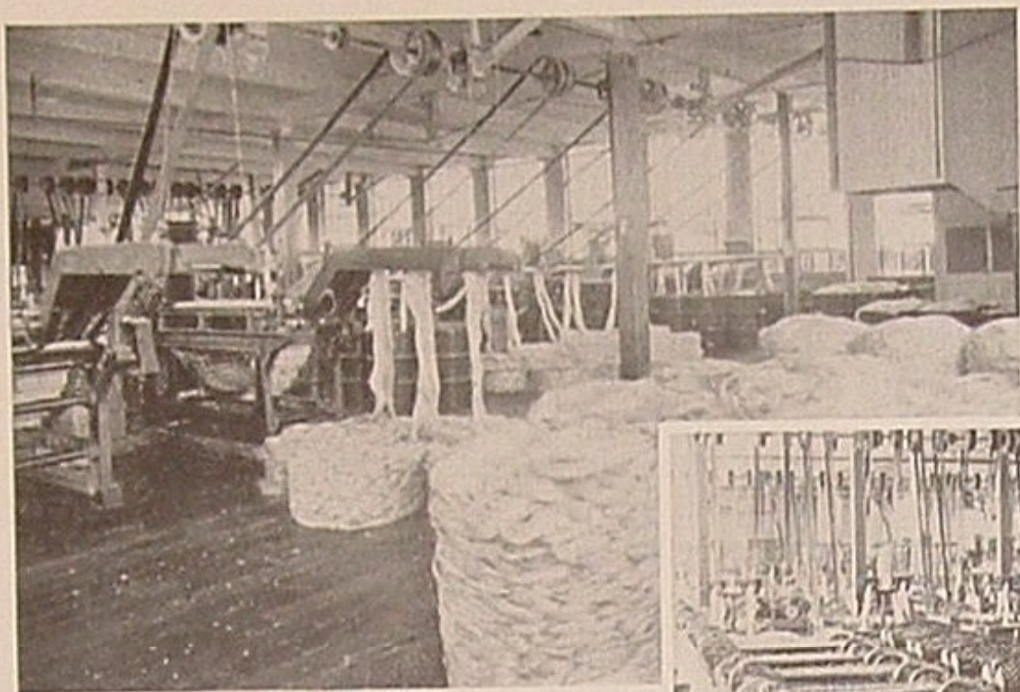
Left: A view of the preparation line at the Great Western Cordage Company plant at Los Angeles. Here the selected and treated rope fiber is made ready for spinning.
