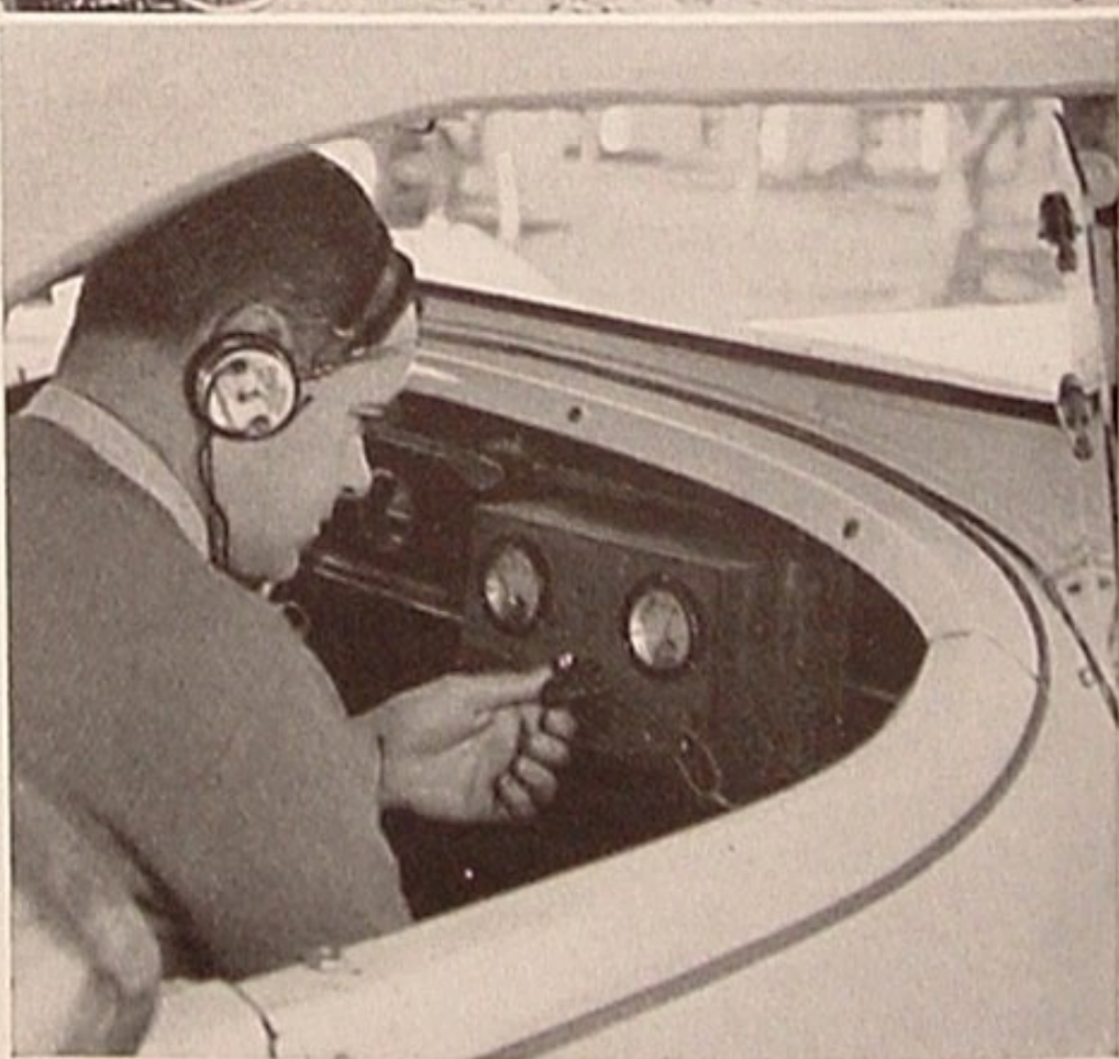
Bottom right: Portable apparatus by which driver was enabled to determine slightest tendency to knock.
