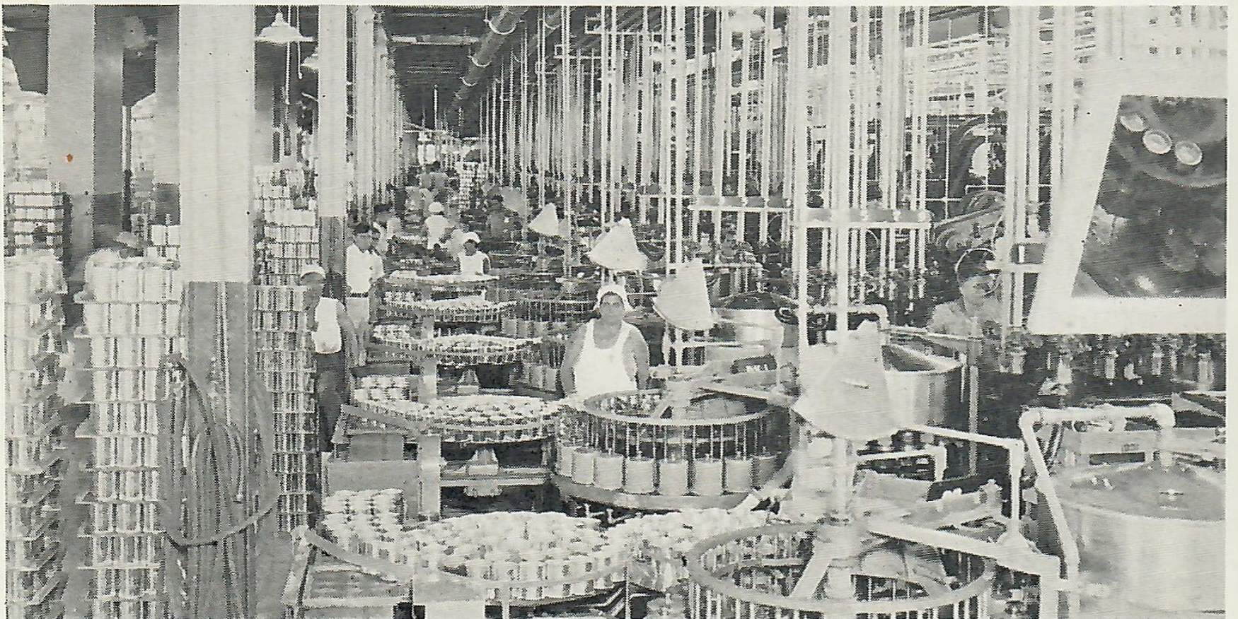
One section of Hawaiian cannery showing sliced pineapple being fed to the pre-vacuumizer machines.
