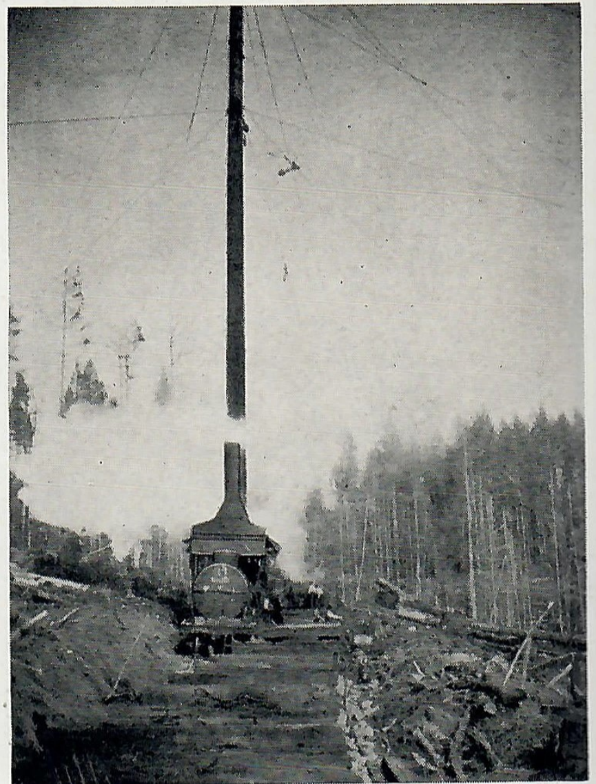
Operating skidder of Andron Logging Company at Mayfield, Wash. Logs are hauled for a mile or two out of the cutting areas with this equipment.
