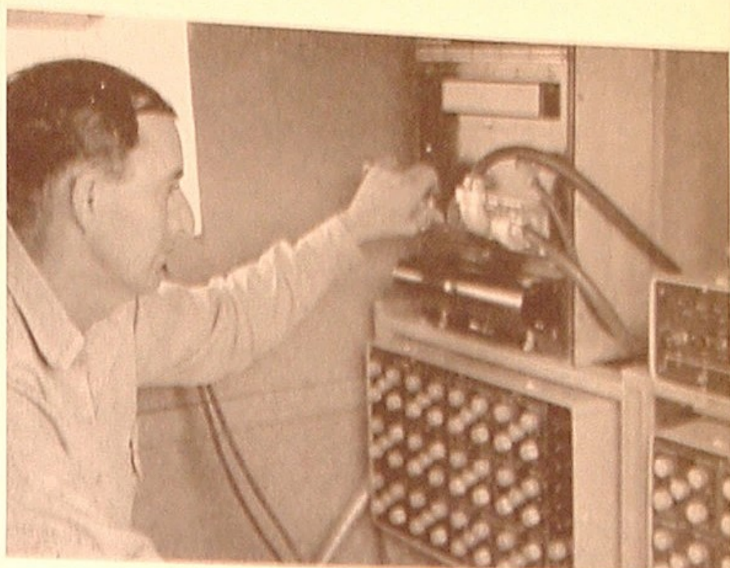
Inside the "dog house," Observer L. D. Driskell checks his camera and amplifiers preparatory to recording the reflected shock waves on a seisogram.
