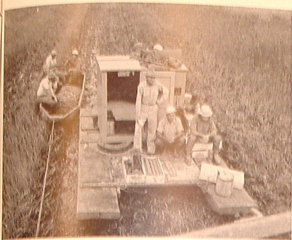
Being towed into position for the next shot is the recording "dog house," also on pontoons. Enroute the "jug hustlers" will pay out half of their cable.
