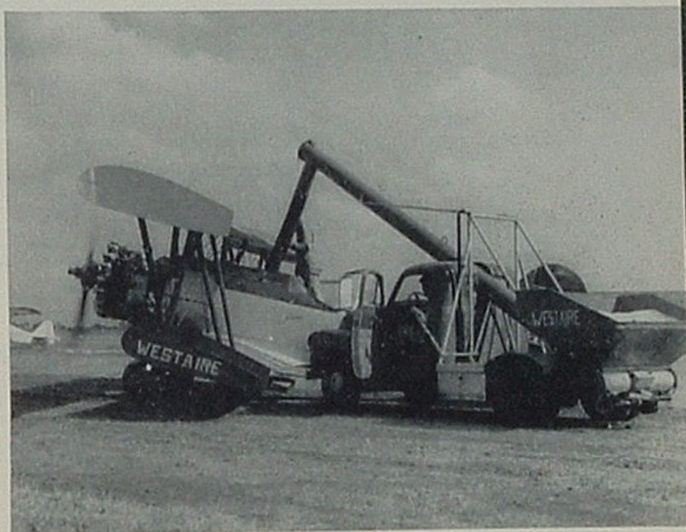
Above, the prills are being conveyed to the hopper of a California "crop duster;" below, the airplane drops its load of fertilizer on a crop thirsting for vital nitrogen.
