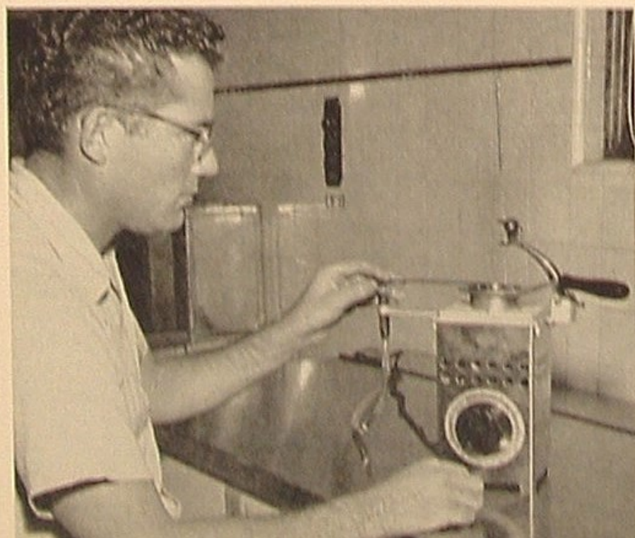
Modern asphalt testing methods in a refinery are demonstrated (above) by Inspector Paul Hougan, using a precision "penitrometer" to measure hardness of a sample; and (below) by Inspector Don Killday, using a Cleveland open-cup flash tester to determine the flash point.
