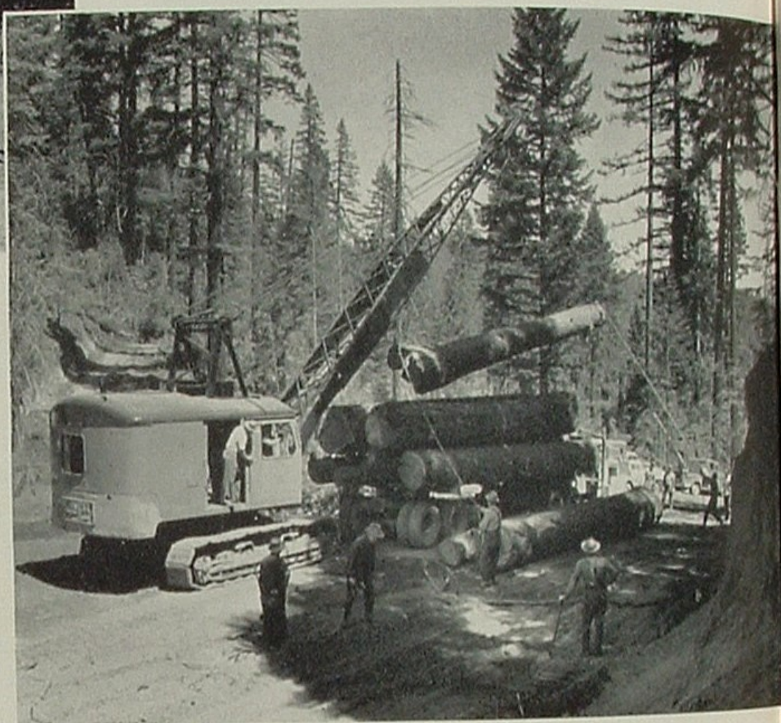
Logs are dragged several hundred feet to the "landing" by winch-equipped "Cat" tractors, left. At the "landing," below, a shovel-loader swiftly loads the logging trucks.
