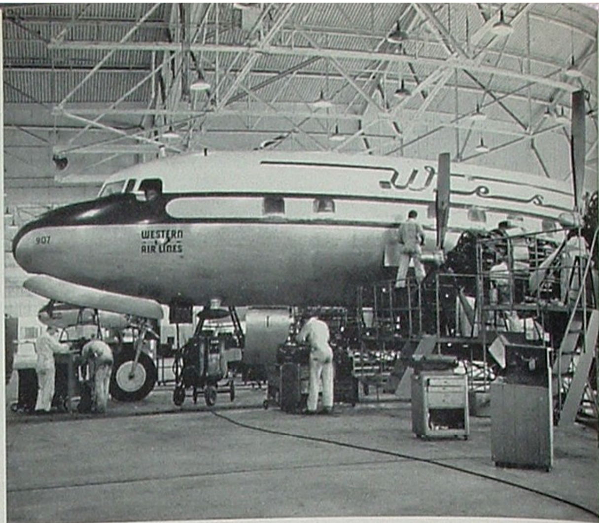
In maintenance and overhaul shops, Los Angeles, all planes are regularly inspected. At 1600 hours the $49,000 engines are removed and completely overhauled.
