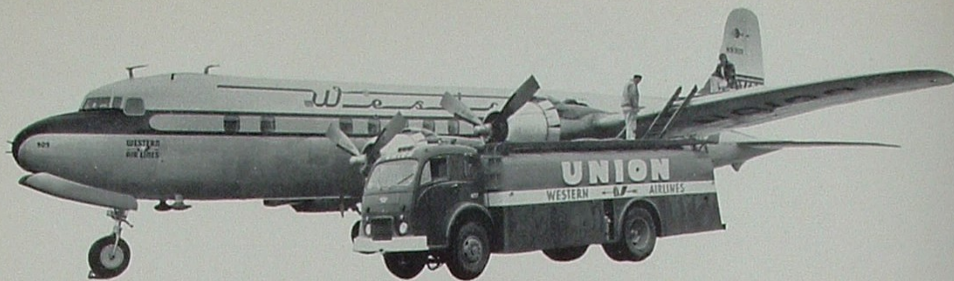
Seven airplane fueling trucks assigned to Western at Seattle, Salt Lake City, San Francisco, Las Vegas and Los Angeles afford easiest fueling and de-fueling of planes.
