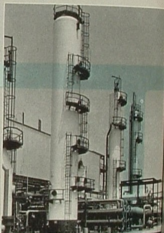
CARBON DIOXIDE REMOVAL is effected by its absorption in MEA solution. Stripped from solution in distillation columns, above, the \text{CO}_2 is compressed and cooled to yield dry ice.
