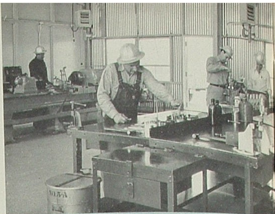
MACHINE SHOP —General mechanical repairs and maintenance on plant equipment are handled by machine shops. The mechanics are shown working on valve assemblies.
