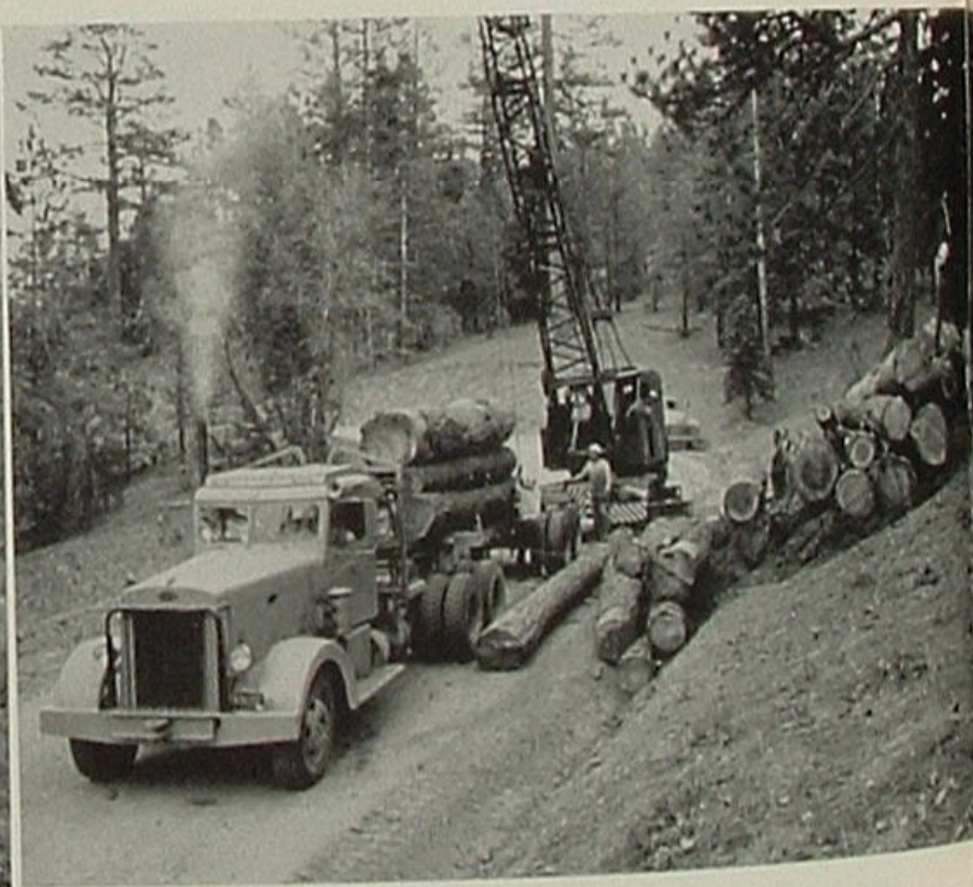
Loading of the logs is done with a diesel-powered crane. Note the use of hard hats by these forest workmen, who take extraordinary care not to cause or suffer injuries.
