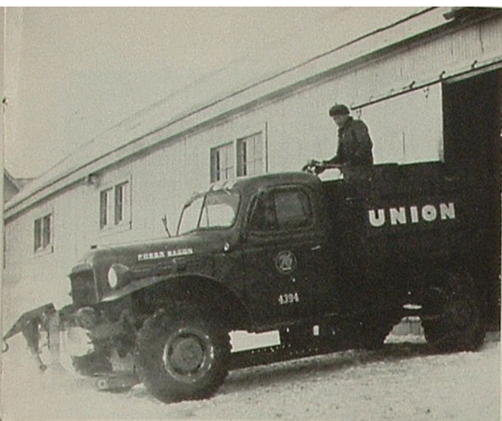
Harold Chappelle's barrel truck at Whittier is geared with a snow plow for bulldozing roadways in and out of the plant yard. The 76 Jeep, below, also shows a few Arctic necessities added to its original factory design.
