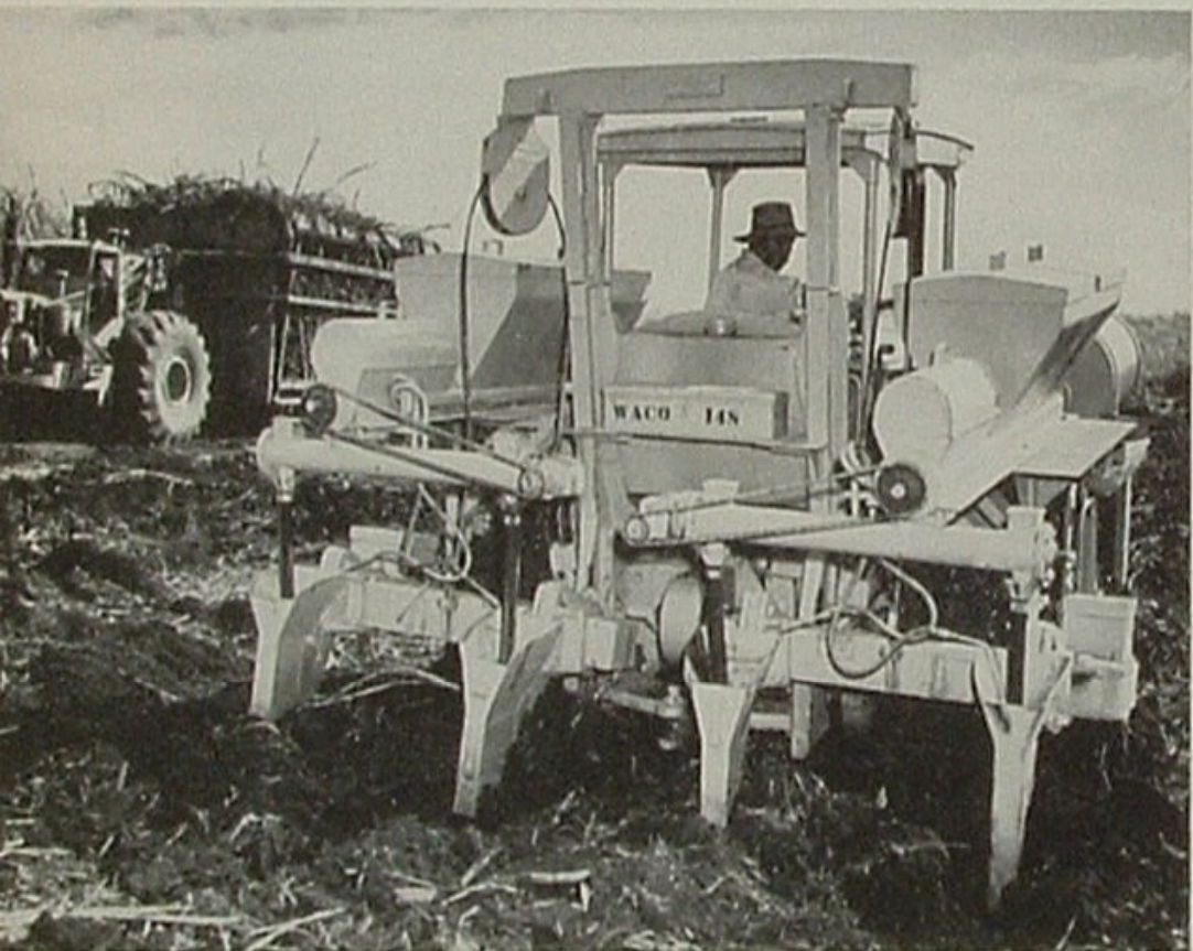
Fertilizing equipment at Waialua plantation carries Brea Aqua Ammonia in tanks, to supply nitrogen, and dry potash and phosphate fertilizers in hoppers. All three basic cane nutrients are applied simultaneously to soil.
