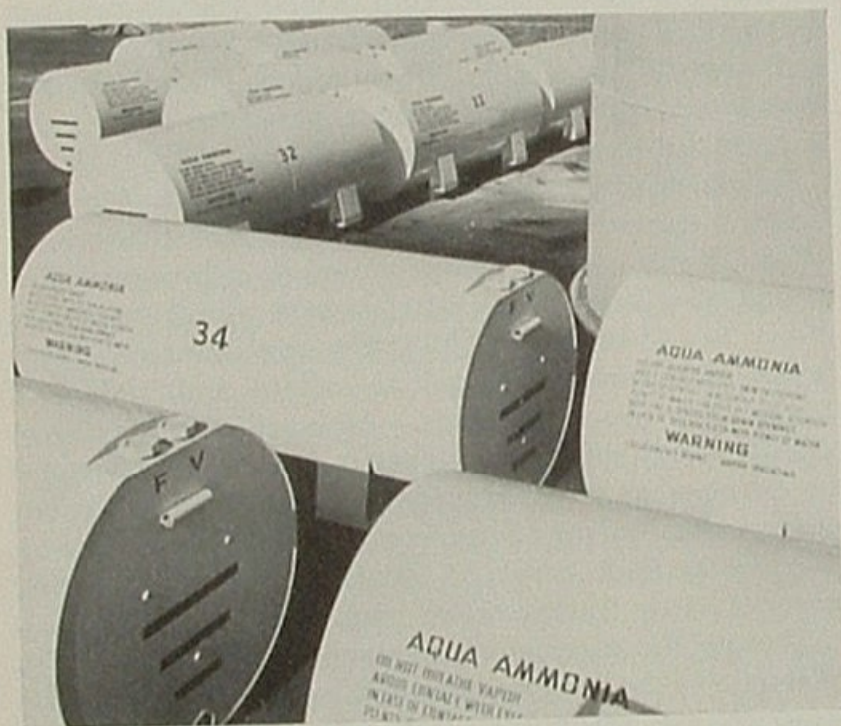
From a storage tank in the factory area at Ewa, aqua ammonia is transferred to field tanks, above. The operator, below, uses mask and rubber gloves during filling operation as safety precaution against irritating vapors.
