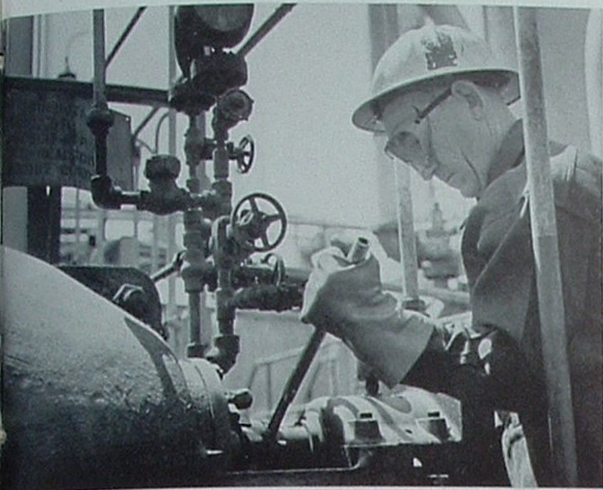
Working on an emulsion pump handling corrosive chemicals, Frank Malovich is protected against acid burns by helmet, monogoggles, rubber gloves and woolen clothing.
