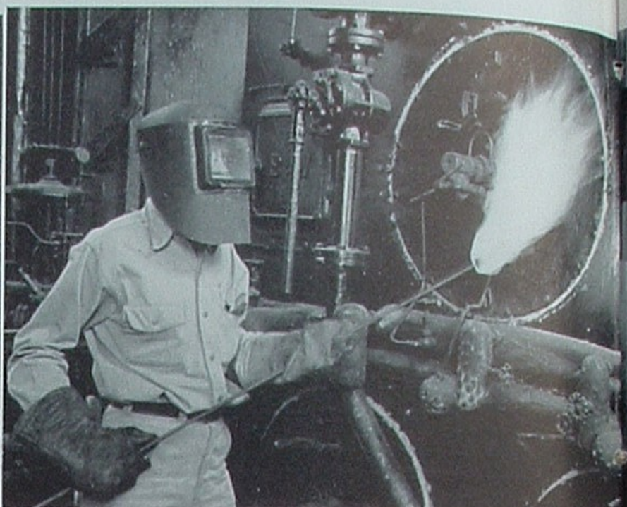
and asbestos mittens while lighting off a furnace fire. Failure of an employee to use the latter precaution resulted in at least one lost-time injury at this refinery.
