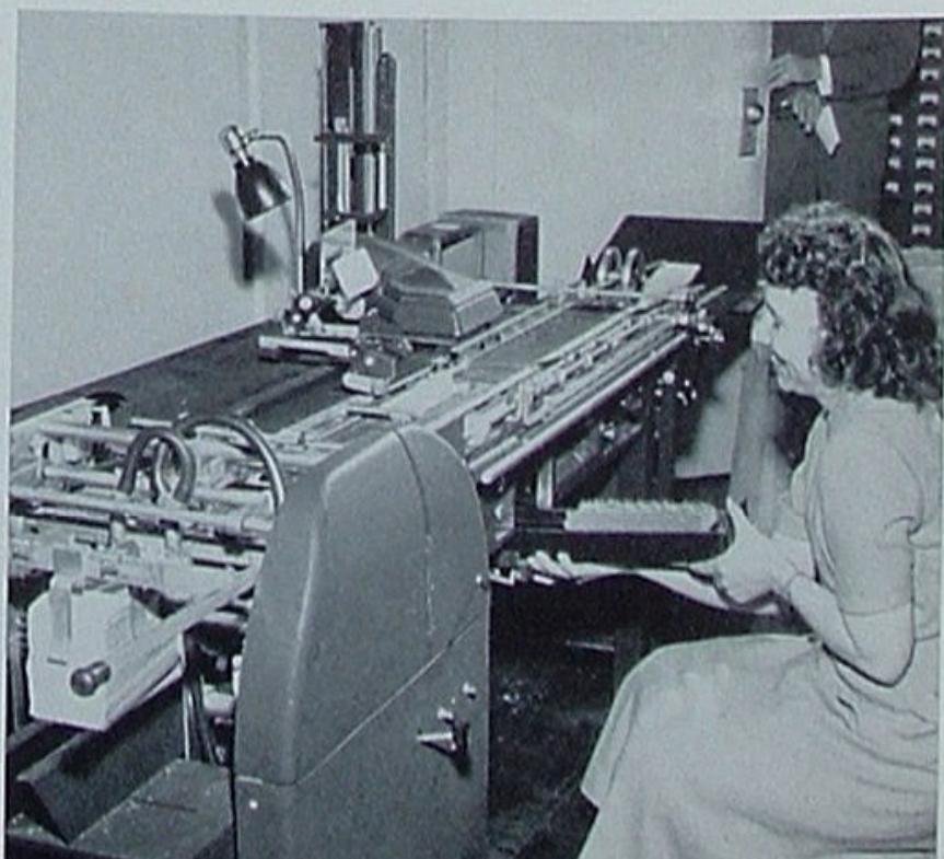
An addressograph machine is kept busy printing monthly statements as well as all quarterly and annual credit cards.
