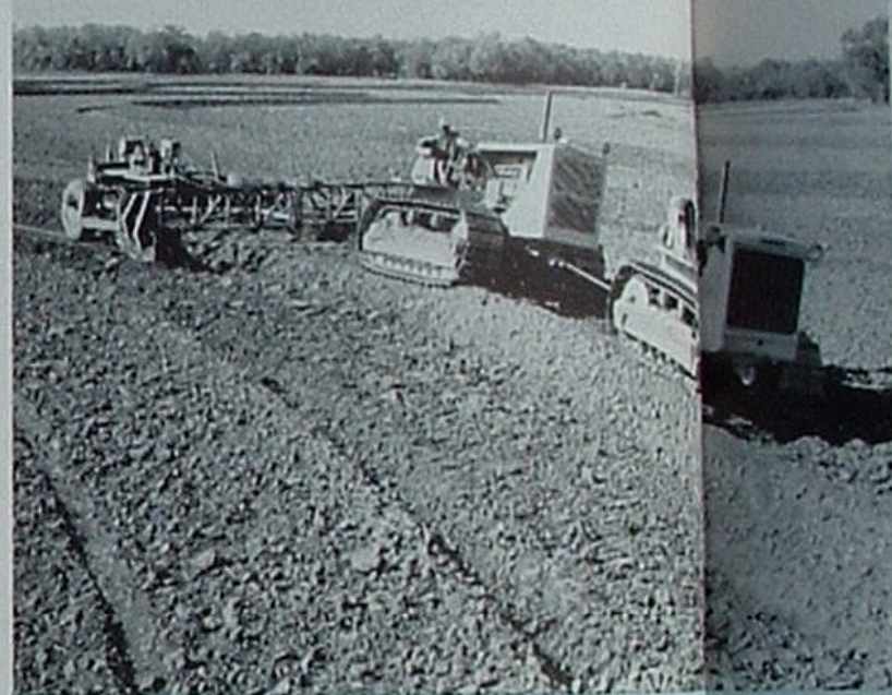
Prior to planting, a rice-checker molds the curving levees, called checks, that partition a rice field into its graceful, water-controlling contours. This one-man-operated grain harvester was designed by the Heidricks in their own shop.
