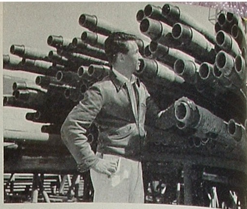
Thomas Stoy, petroleum engineer trainee, examines the stack of drill pipe that penetrated 6,099 feet of earth to complete Jewett Fee No. 83, producer on this month's cover.
