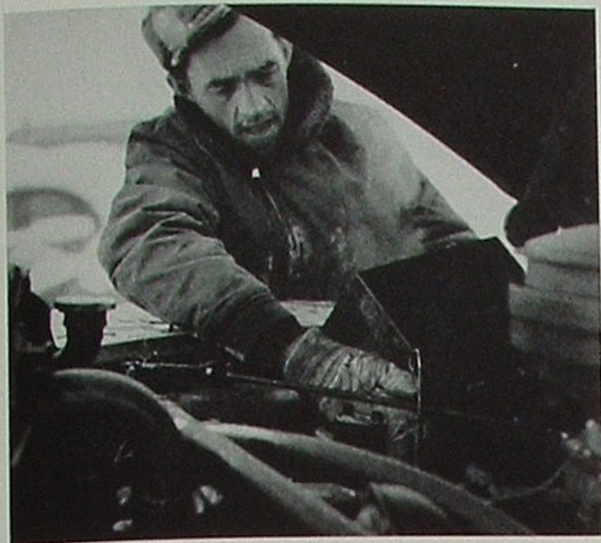
At temperature of minus-50 or colder, even batteries have to be protected against frost damage. The Ohioans learned to handle such chores with their mittens on.
