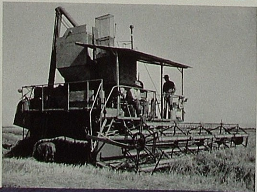
Harvester combines enter the rice checks in October. They thresh the grain and accumulate a truckload in top hopper.
