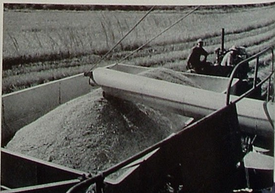
Tractor-drawn "bank-out" wagons receive the load of threshed rice and take it across muddy fields to a road.
