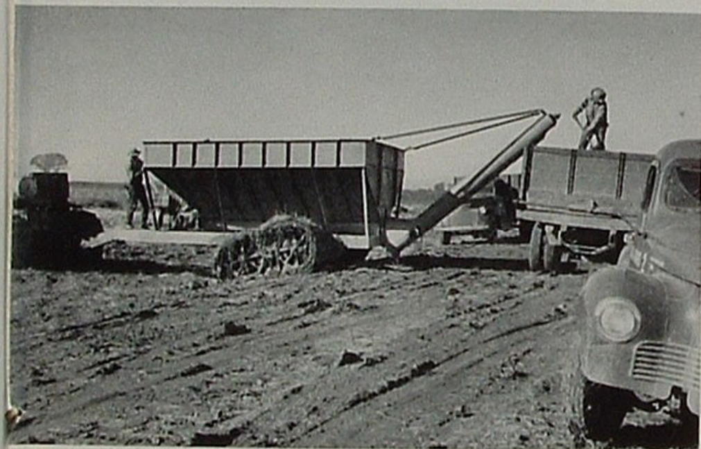
Bank-out wagons are emptied mechanically by gasoline-powered screw conveyor into conventional grain trucks.
