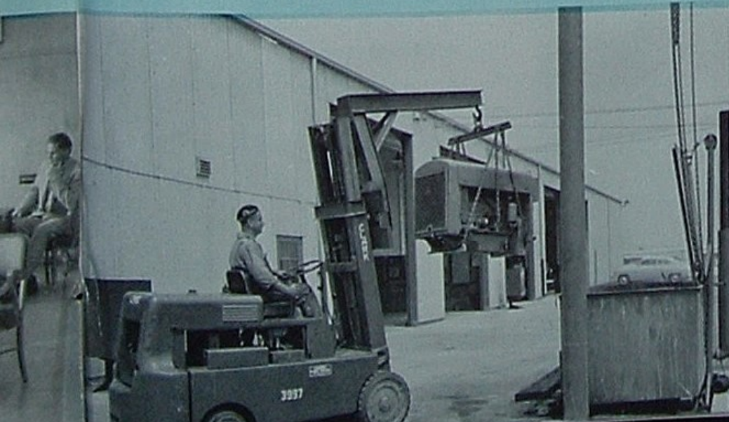
Below, Mechanic "Frenchy" Lacoste shows newest method of lifting heavy engine into hot Oakite bath tank, right.
