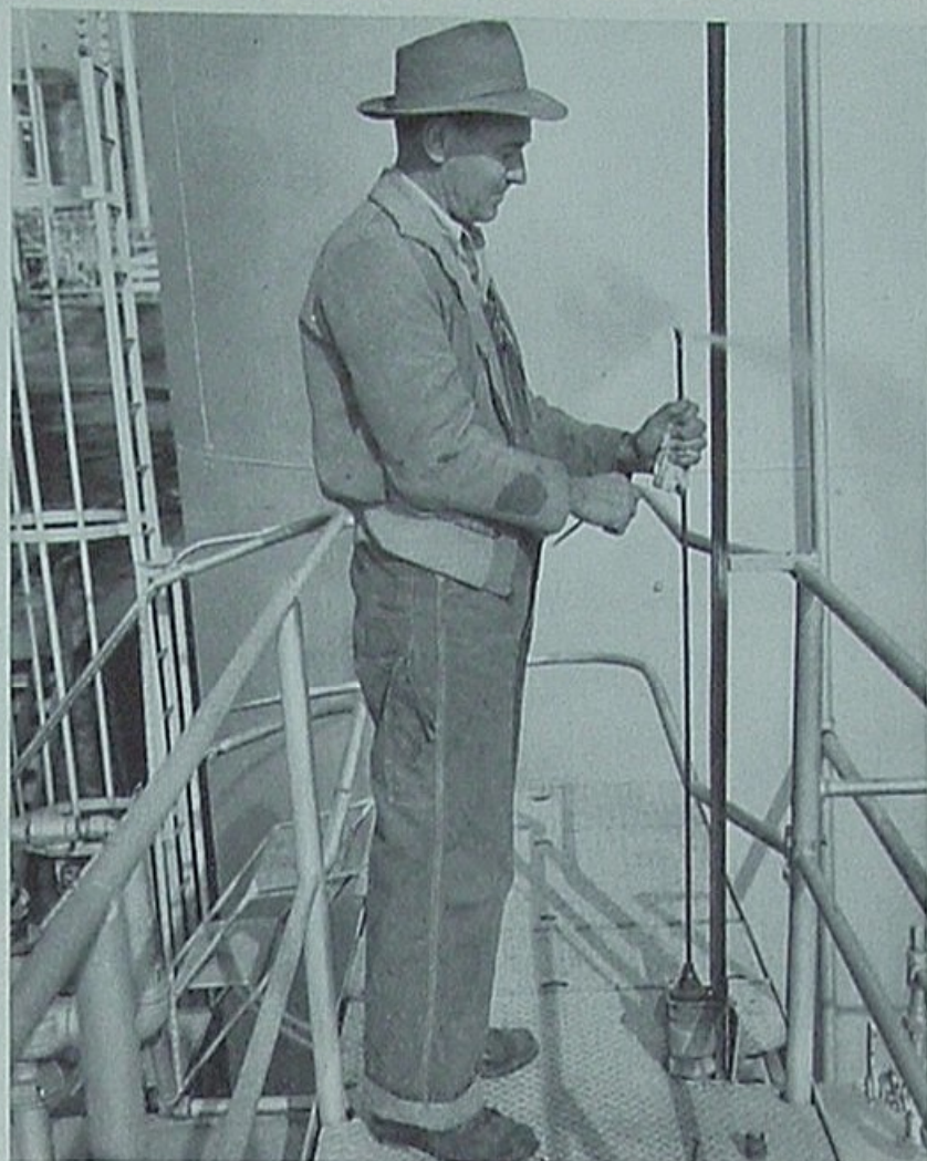
Gauging propane storage is J. R. Salvage, plant operator. Propane gas emerging from the vent hole indicates that the gauging tube has reached level of compressed liquid.
