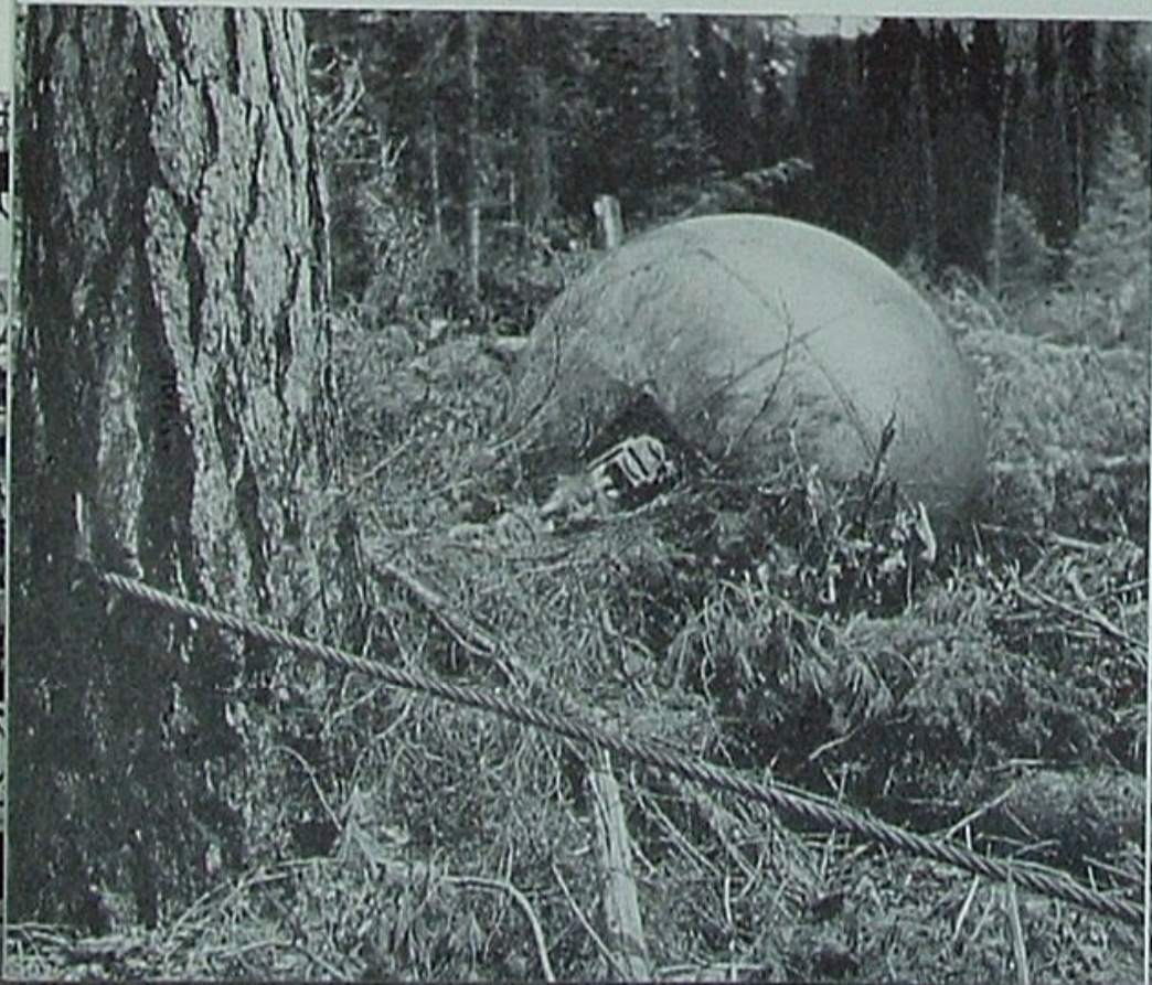
The steel ball's special functions are to carry taut cables over old logging stumps and give tractors a four-foot high leverage on big trees to facilitate this uprooting technique.
