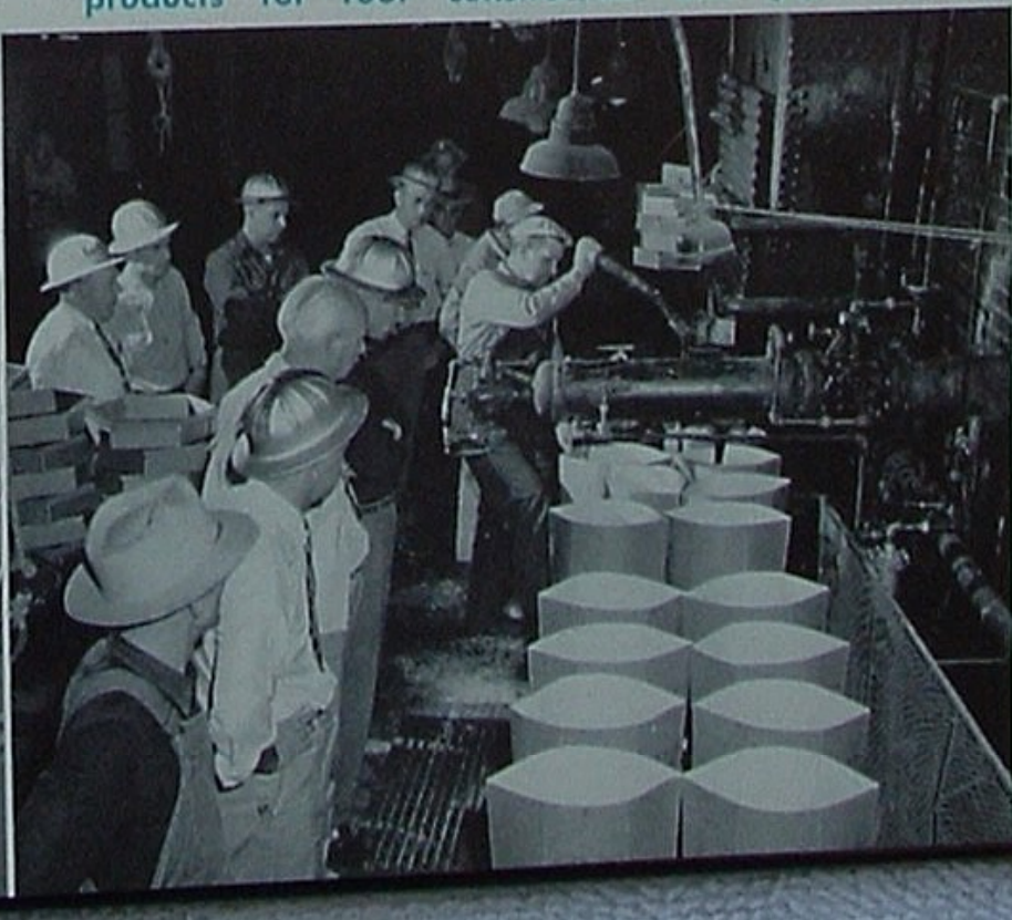
In Oleum's Asphalt Department, the group observes techniques used in filling hex-cartons two at a time with products for roof construction and pipe coating.
