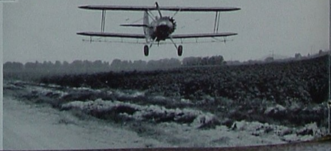
(Above) Liquid spray is often mixed near the field of operations, then pumped by auxiliary unit into hopper. (Right) At such low altitudes, the propeller-wash thoroughly stirs liquid or dust spray into an infested crop.
