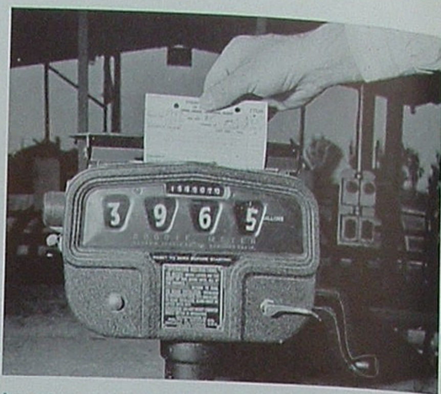
Ingenious meters, said to be the largest ever installed, measure each load of gasoline and record gallonages on truck loading tickets with this printing mechanism.
