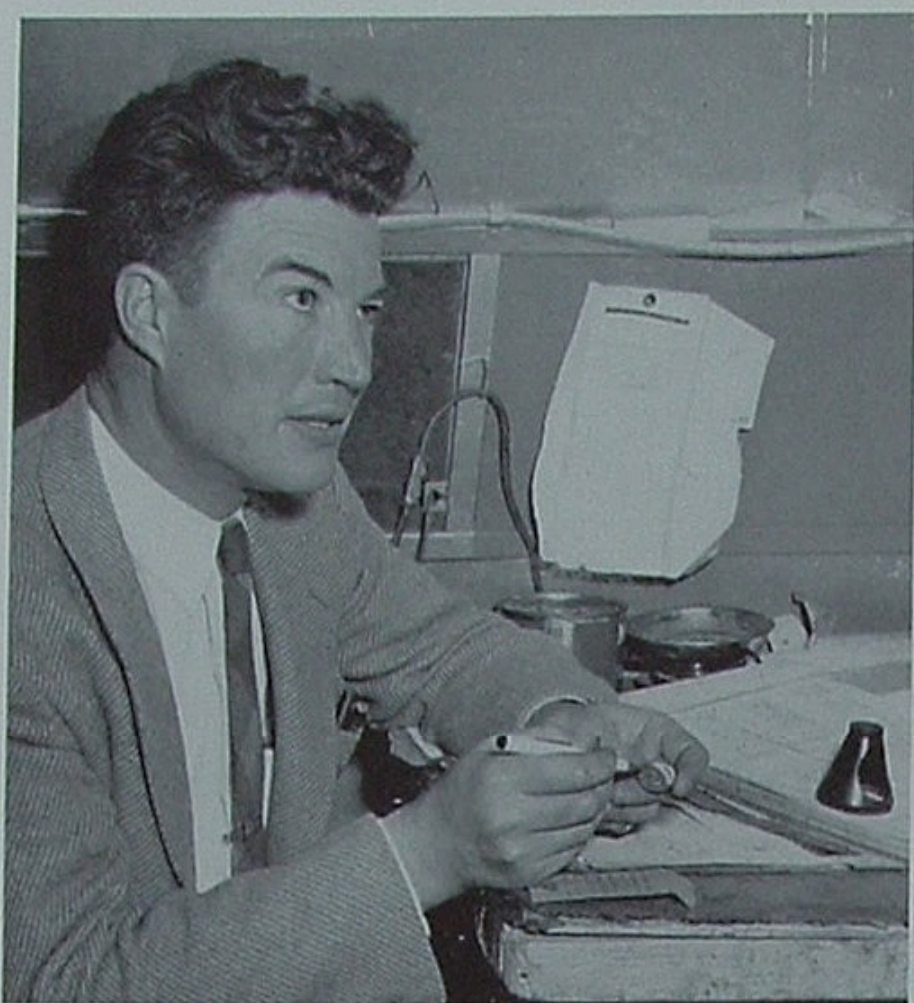
From a single-shot survey picture taken deep underground Tal Ledbetter, division drilling foreman, ascertains whether or not the crew is drilling a straight hole.
