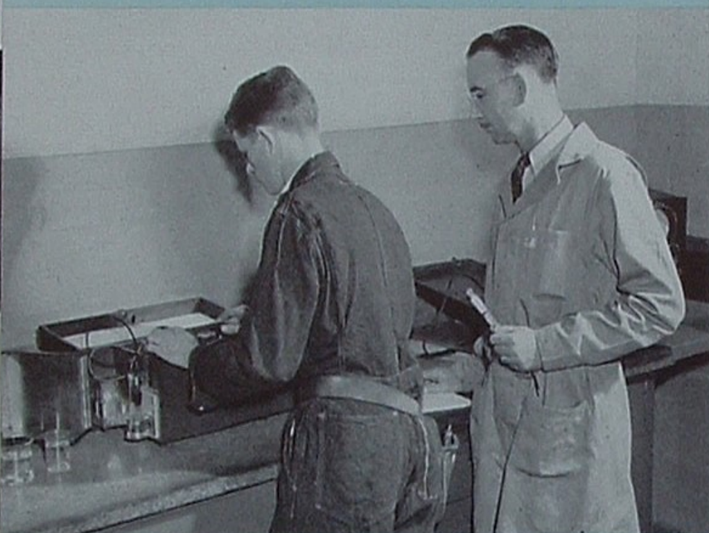
Ralph Apel, left, and Foreman Robert Cakebread use portable test equipment to determine the pH (acidity-alkalinity) content of sample.
