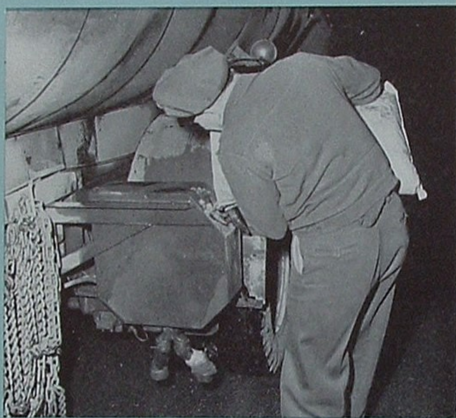
Mountaineering transports in Washington are equipped with sanders for supplying traction in case of emergency stops on icy roads.
