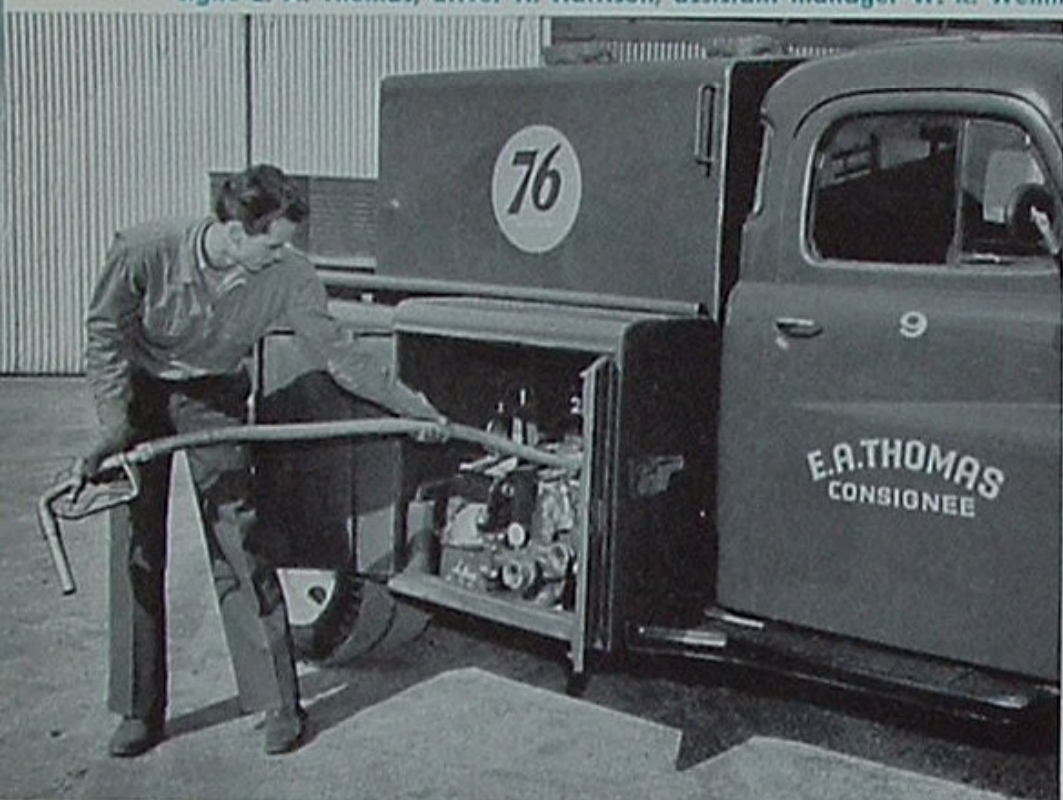
Highly versatile trucks with meters, pumps and hose reels carry mixed loads of bulk fuels and packaged lubricants to customers.
