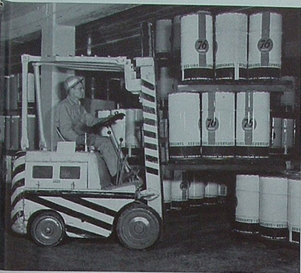
With this 4000-pound capacity "Jitney" Raymond Sampson can fill or empty a large warehouse in less time than several men once required.
