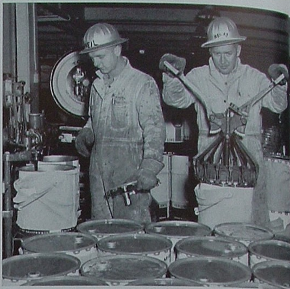
While Neil Bachman feeds 30-pound pails to an automatic weighing and filling machine, A. J. Henry seals pails with a lid crimper.
