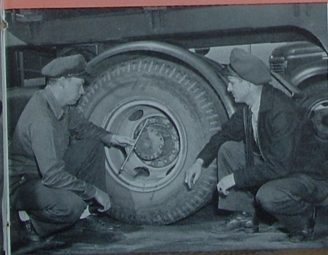
Checking tire pressures at change of shift are transport drivers Stanley Smithem, left, and William Carman. This and other precautionary checks prevent many an accident or a breakdown on such busy thoroughfares as Eastshore Boulevard, right, where stopping would be risky.
