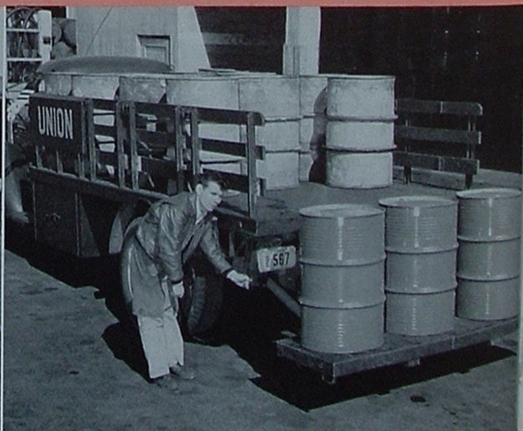
Left: Driver George Carman and loader Rene Lorette compare dome and meter compartment commodity tags to prevent delivery of, say, gasoline into a cleaning solvent tank. Right: James Hendryx demonstrates how the hydraulic tailgate lessens physical hazards of barrel handling.
