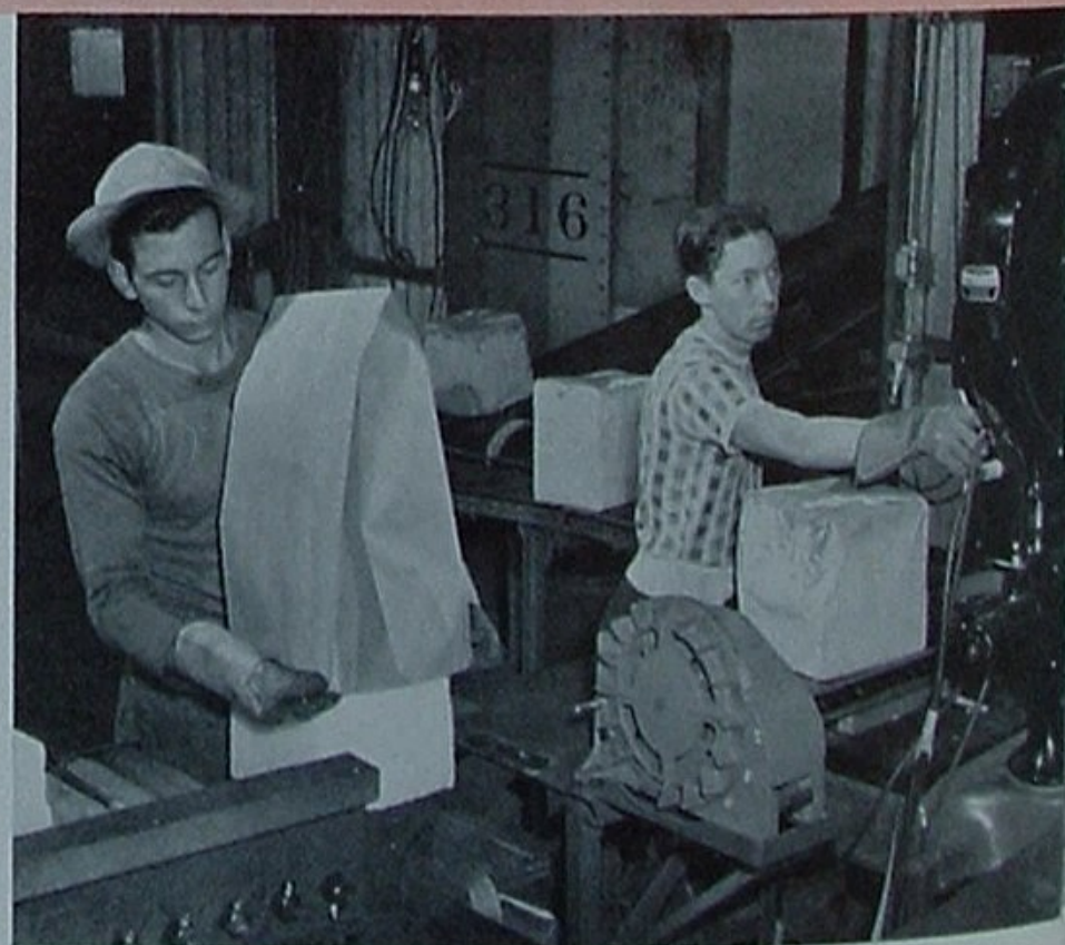
Packaging consists of slipping a paper bag over each cube and tape-sealing the open end. After being weighed, the blocks proceed via conveyor belt to car. Workmen are (l-r) F. Goodchild and D. Foster.
