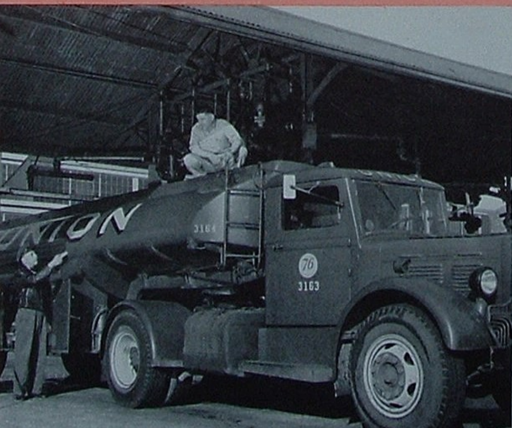
Left: Driver George Carman and loader Rene Lorette compare dome and meter compartment commodity tags to prevent delivery of, say, gasoline into a cleaning solvent tank. Right: James Hendryx demonstrates how the hydraulic tailgate lessens physical hazards of barrel handling.
