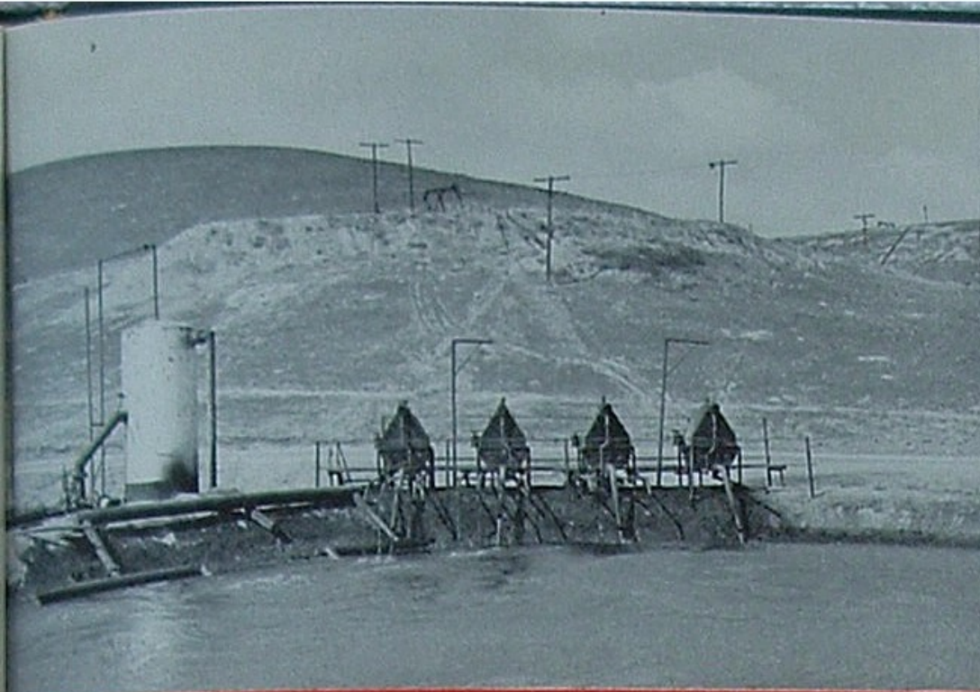
From 42 wells on the S & M Lease, oil and water mixtures flow through these four weigh meters into the open sump;
