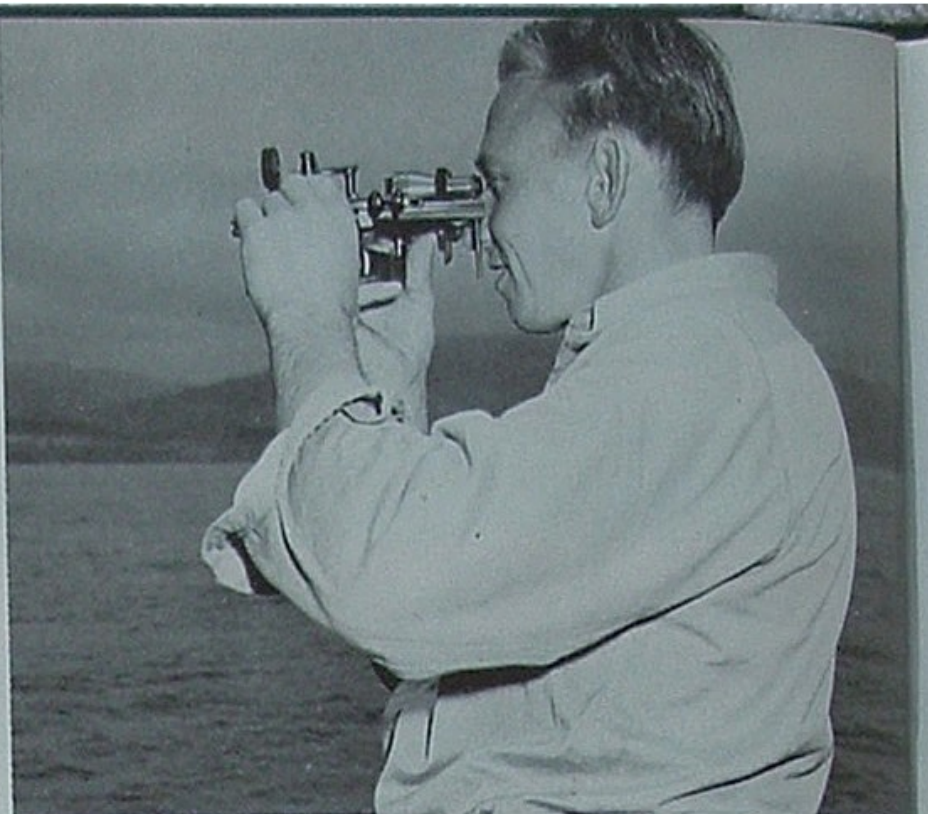
A party member measures angles to established landmarks in order to fix the exact location of each ocean-bottom sector explored.
