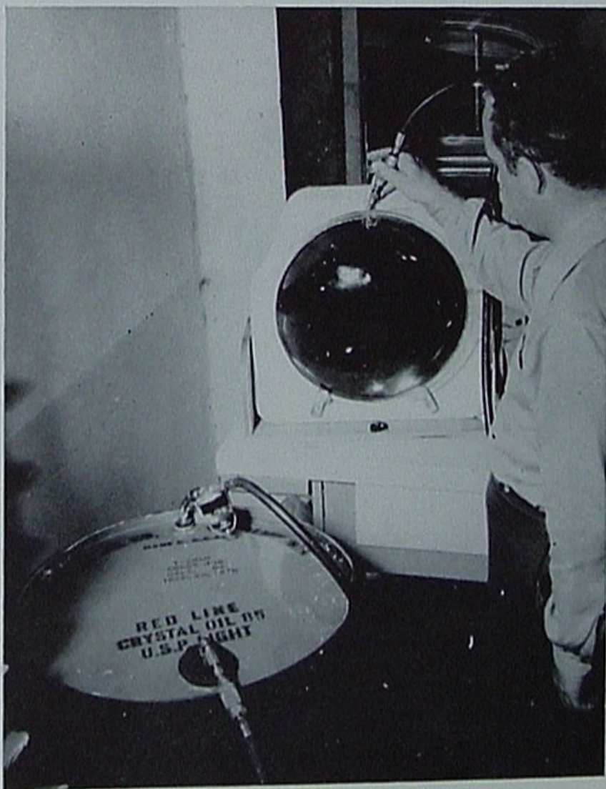
This is how Red Line Crystal Oil is placed between two pieces of plexi-glass to form an excellent television magnifier.
