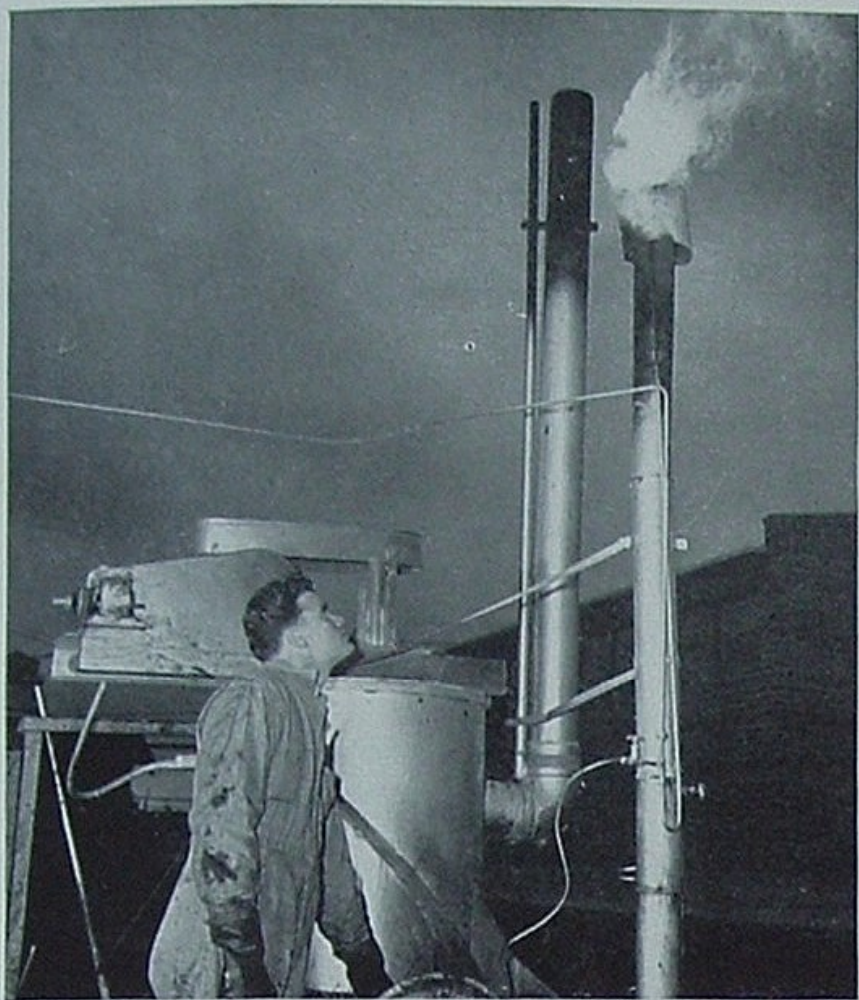
Carbon in the oil shale supplies more than enough heat energy for the retorting process. W. N. Silvis is seen regulating release of excess heat that could be converted into electricity.
