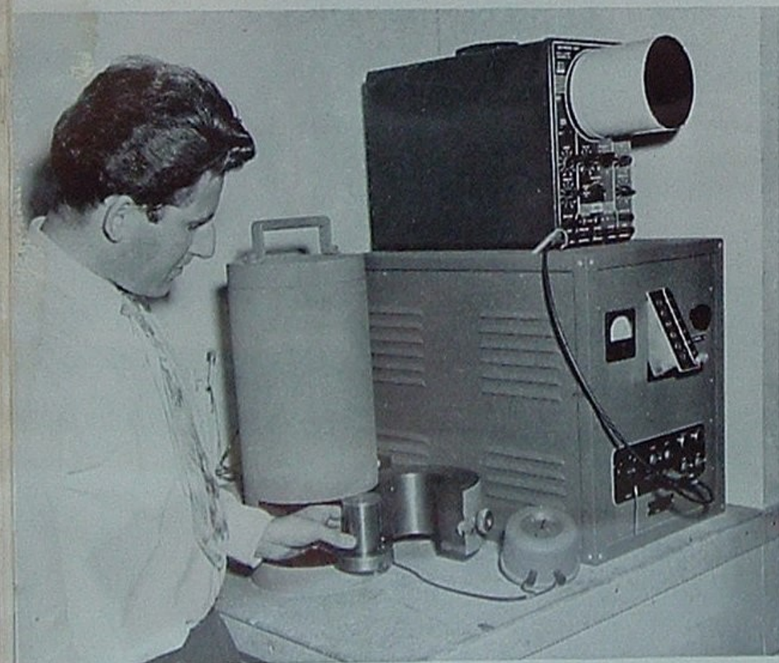
Paul Nahin, research chemist who received his nuclear training in the shadow of a Berkeley cyclotron, places a radioactive sample in lead shield preparatory to counting its rate of disintegration. The "scaling" device at right counts and records atomic radiations.
