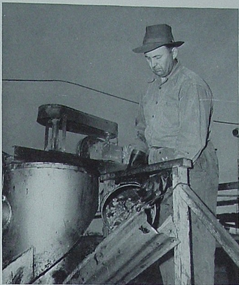
The method here being used by John P. Davis, pilot plant technician, in feeding oil shale into the retort will certainly bow to more advanced techniques when and if a commercial plant is built.
