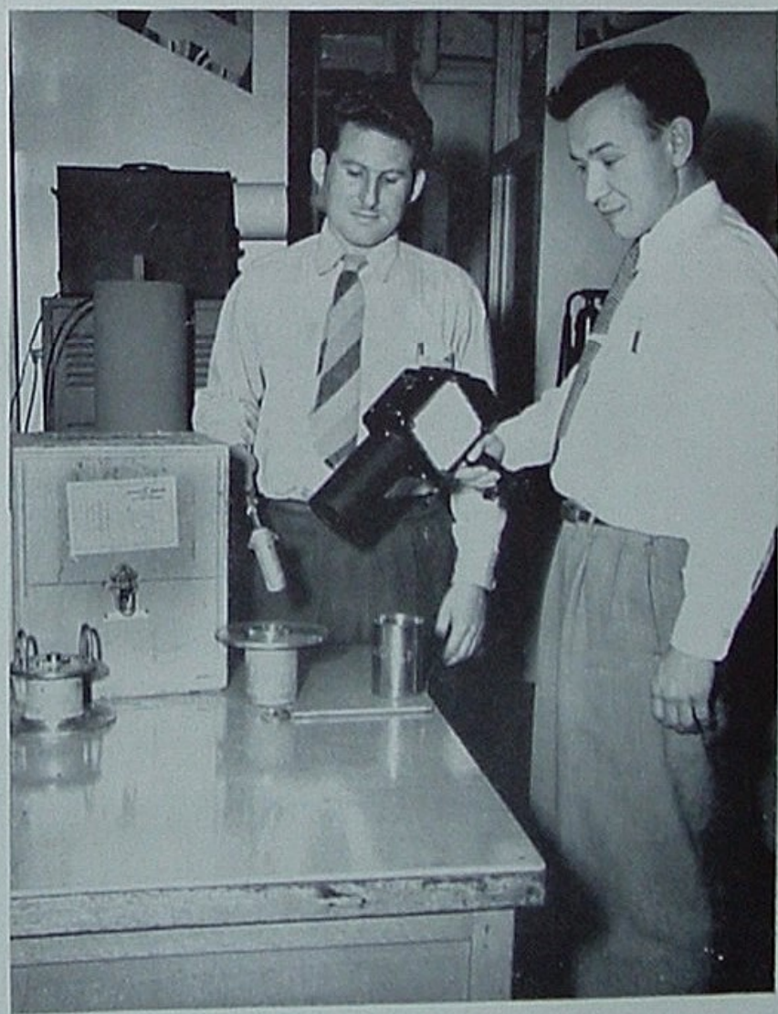
The small aluminum tube just removed by Paul Nahin, left, and Ted Nowak from the comparatively huge shipping case contains less than a teaspoonful of isotopes. The "Cutiepie" held by Nowak is an ionization meter used to detect physically harmful radiations.
