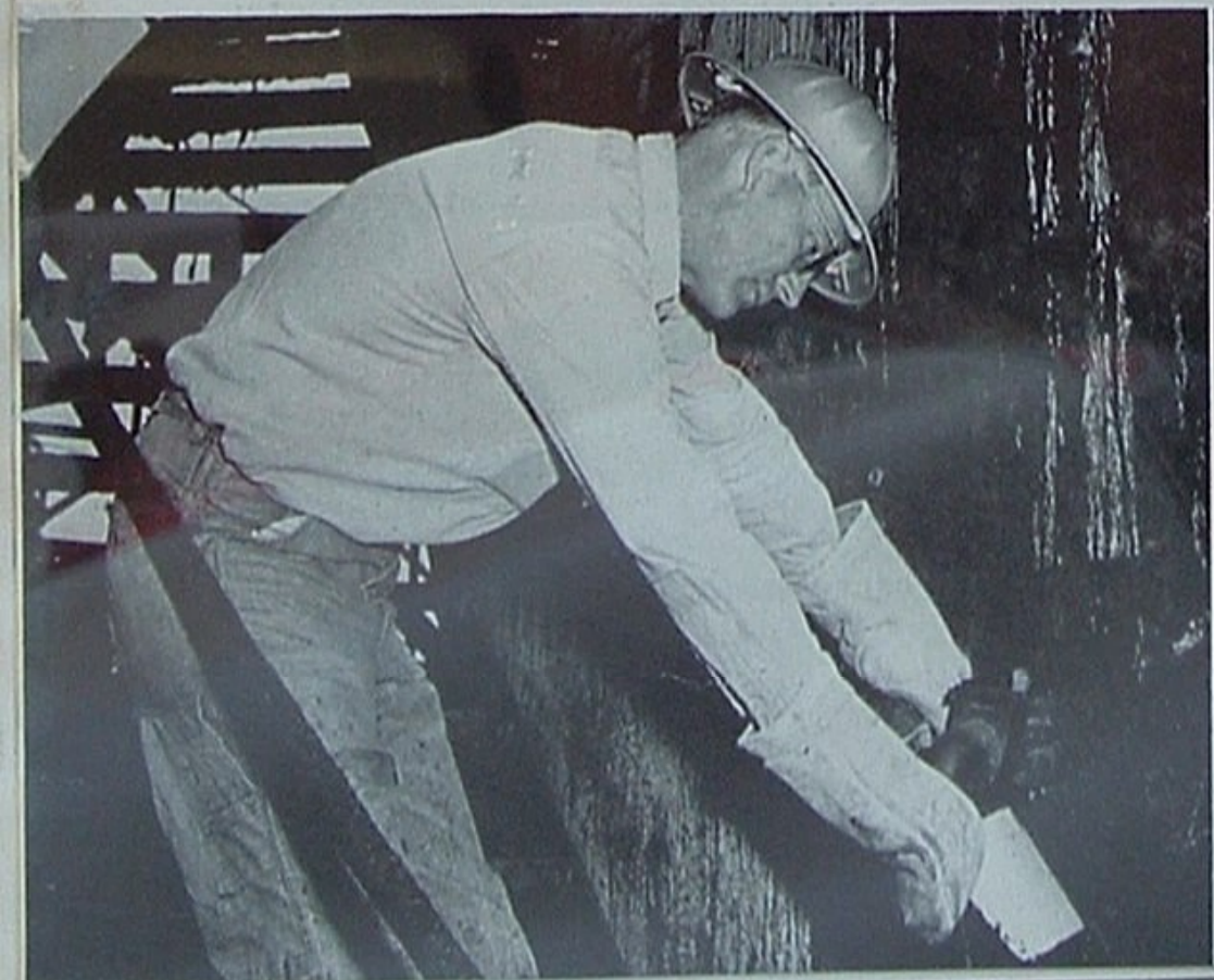
Safety precautions and practices are very much in evidence here as Albin Romansky, left, and Al Maris, sheet metal journeymen in the Tin Shop, spot-weld a new safety guard for a power saw.
