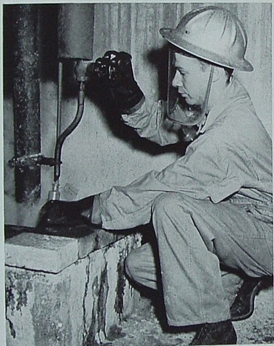
Above: Stillman Sidney Horton takes no chances while drawing sulphuric acid samples from a primary settler. His face shield, hard hat and rubber gloves are insurance against burns and blindness. Right: It was this type of saw blade in this machine doing this kind of work that ended the story. The saw blade broke; an employee's eye was cut; and not a Refinery soul was made happy thereby.
