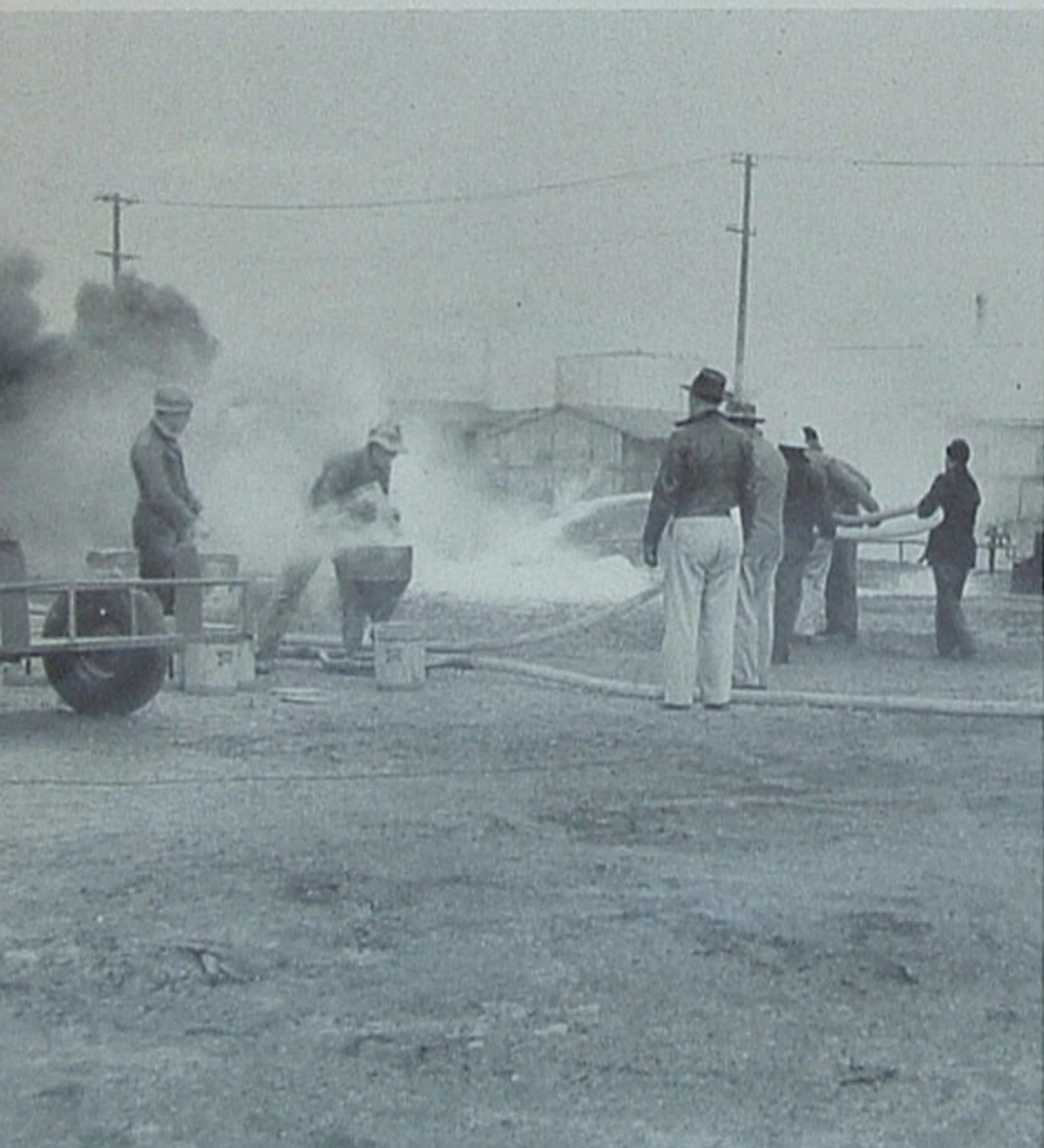
Trainees at Oleum Refinery are using foam to solve this fire problem. The hopper and other equipment in the foreground mix the dry chemical with water, eliminating the need for large storages of chemicals in solution.
