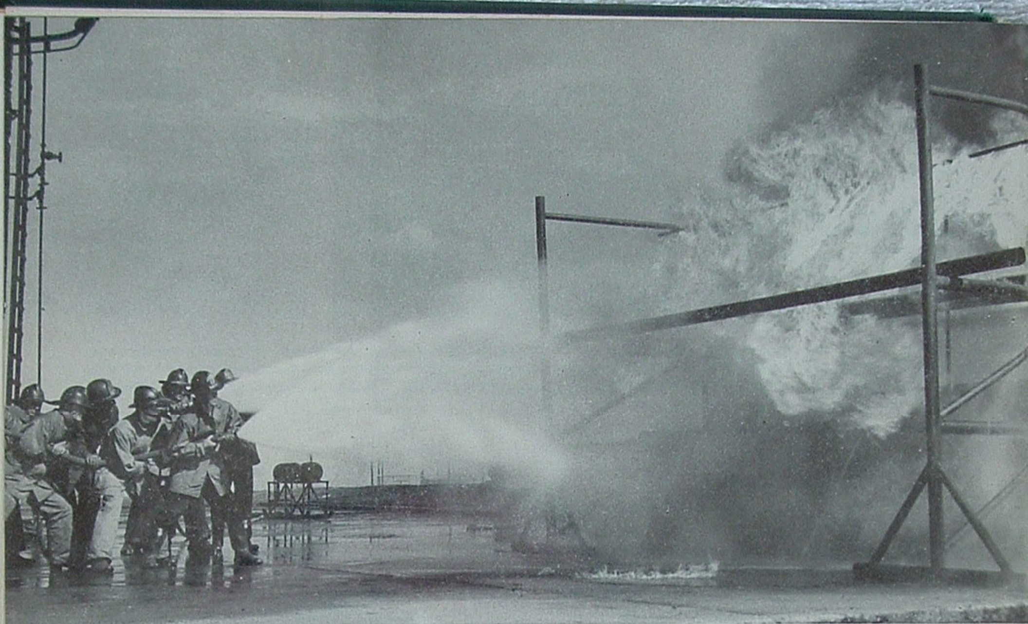
Firemen from the Los Angeles Fire Department try large fog nozzles against a most stubborn type of oil blaze. The prop was engineered to produce a nearly unextinguishable fire. It teaches the problems and techniques of control.
