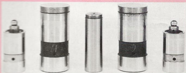
Actual non-rusted engine parts after severe rust test
