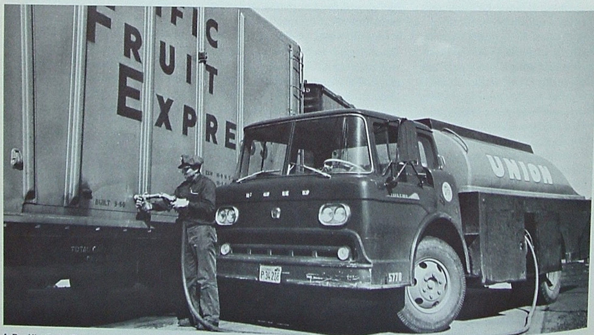
A Pacific Fruit Express refrigerator car uses up to 400 gallons of diesel fuel.
