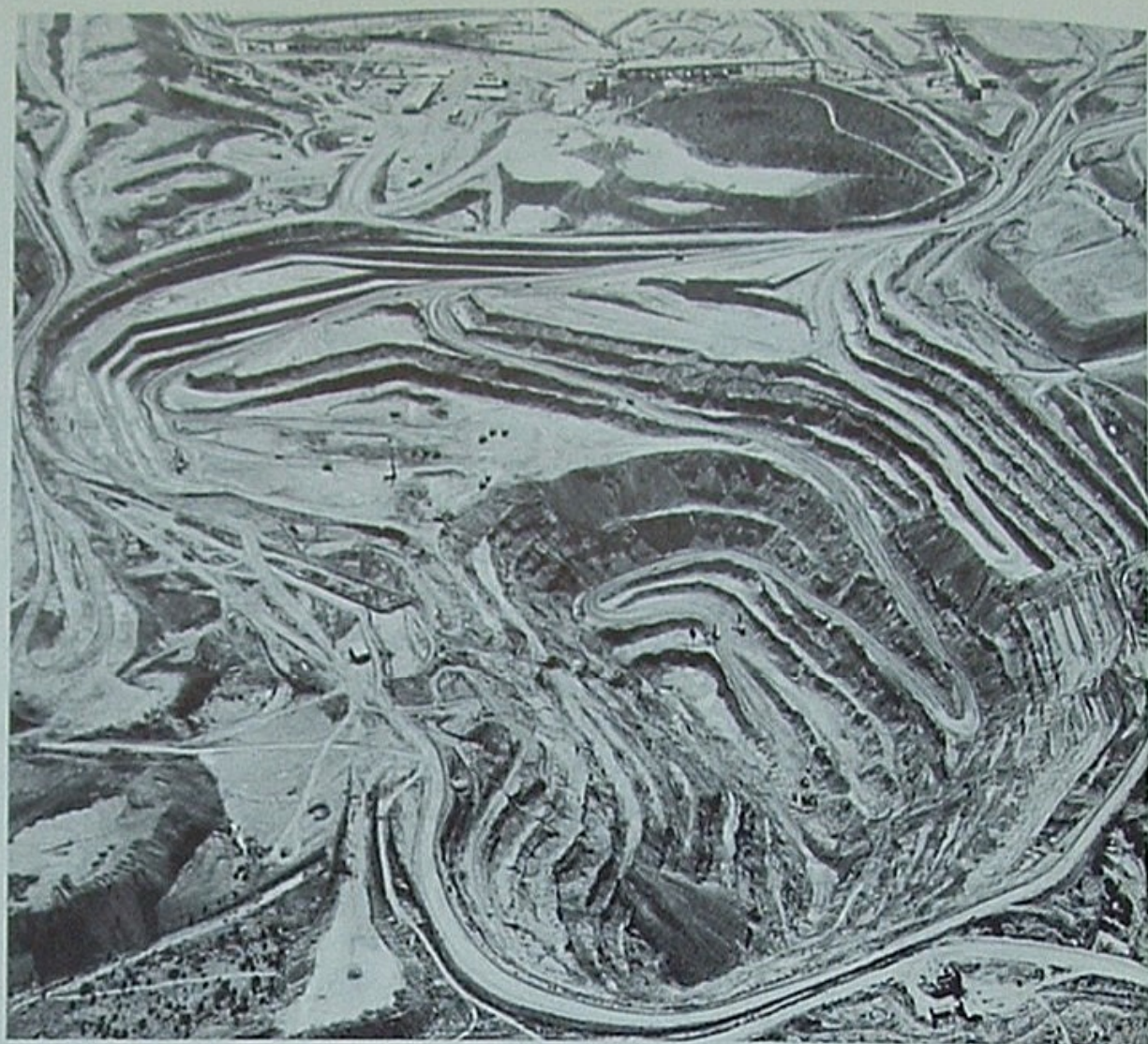
$16 MILLION HOLE. Pima Mining Company of Tucson, Arizona, will spend a projected $16.6 million to expand its operations. The pit is presently 600 feet deep. Plans call for it to be deepened to 1,200 feet. The expansion is forecast to increase the output of copper ore to some 30,000 tons per day. Union Oil owns 25 per cent of Pima Mining.
