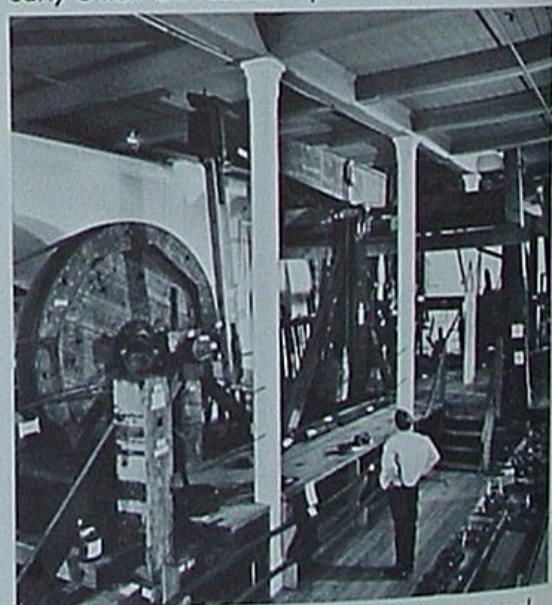
Special attraction is old cable-tool rig, restored inside the museum — minus the original derrick.
