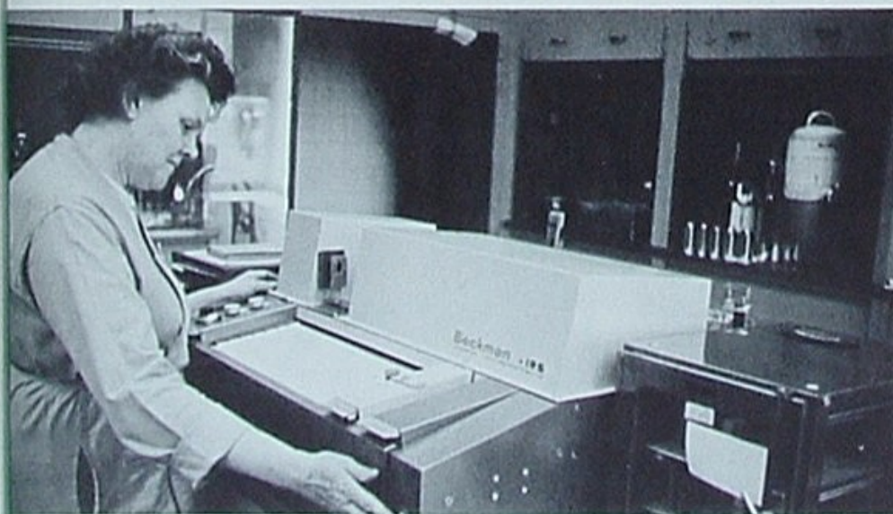
In the chemistry laboratory at Oleum Refinery in the Bay Area, Mrs. Betty Kimmich uses an infrared spectrophotometer to identify the presence of certain molecules characteristic of polymers (plastics).
