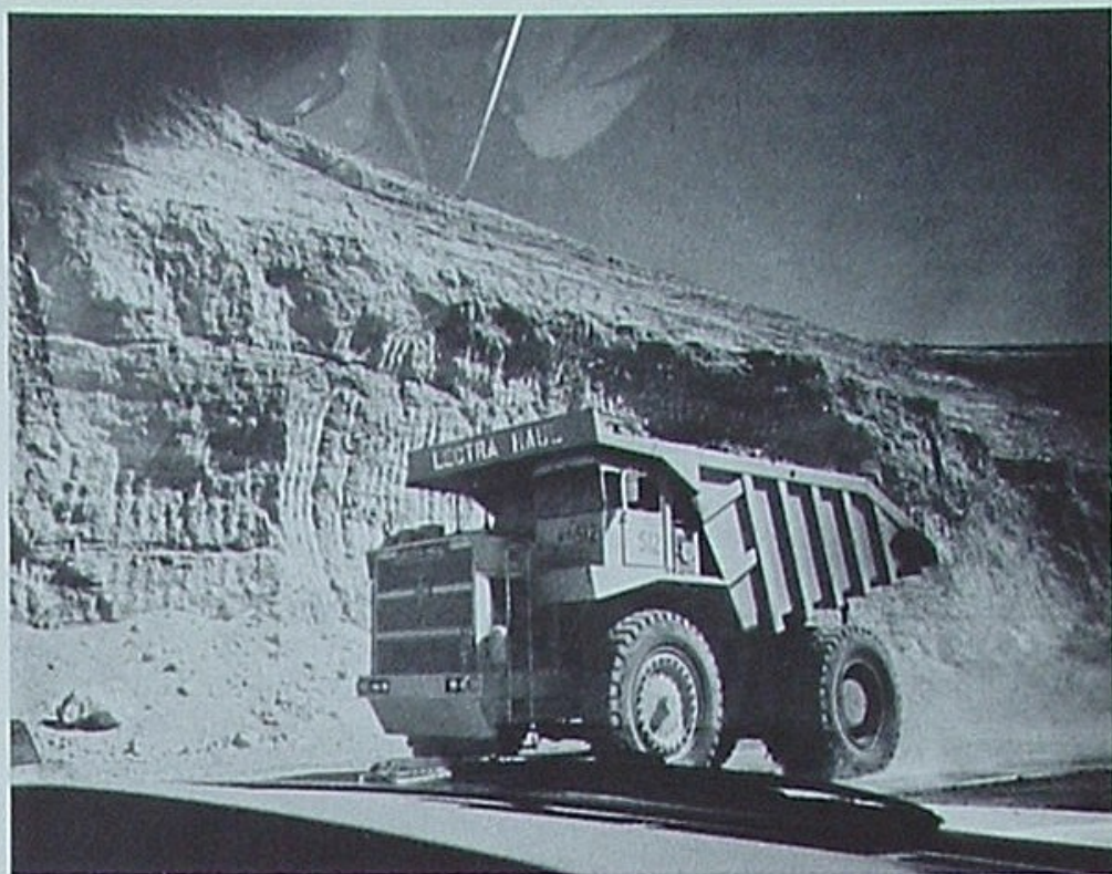
Loaded truck rumbles up 1½ per cent grade at 30 m.p.h.
