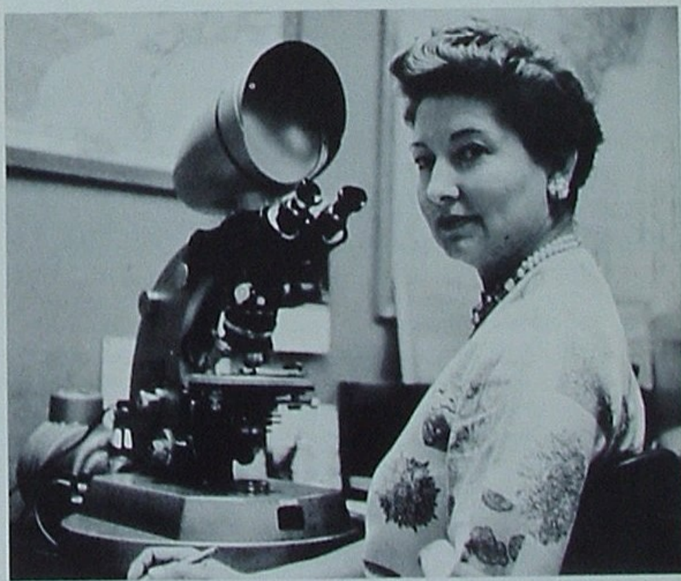
Petrographic specialist Juanita Schmidt of Research Department uses a photomicroscope to identify minerals in core samples of rock. Samples are shaved as thin as 1/1000 of an inch.
