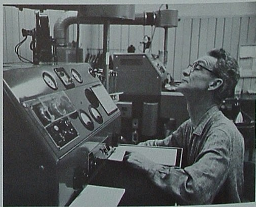
QUALITY: Gasoline must meet rigid specifications. Stanley D. Chapin, inspector at Oleum Refinery, tests for octane number.
