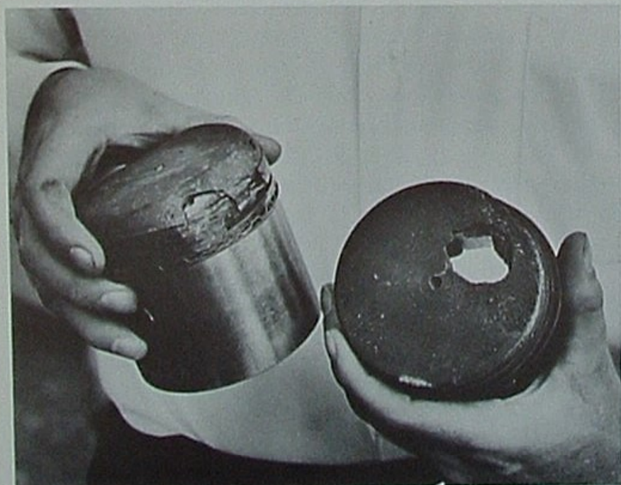
DAMAGE: This isn't likely to happen, but it could. Severe cases of preignition have destroyed an aircraft engine in seconds.
