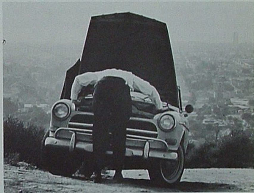
VAPOR LOCK: Suppose you're driving along a freeway or up a steep mountain on a hot day. You slow down or stop and suddenly your engine stalls. You may have vapor lock. What has happened is the light compounds in your gasoline have boiled off in the fuel pump, and the vapors have choked off the fuel supply to your engine. Next time fill up at a Union Oil station.
