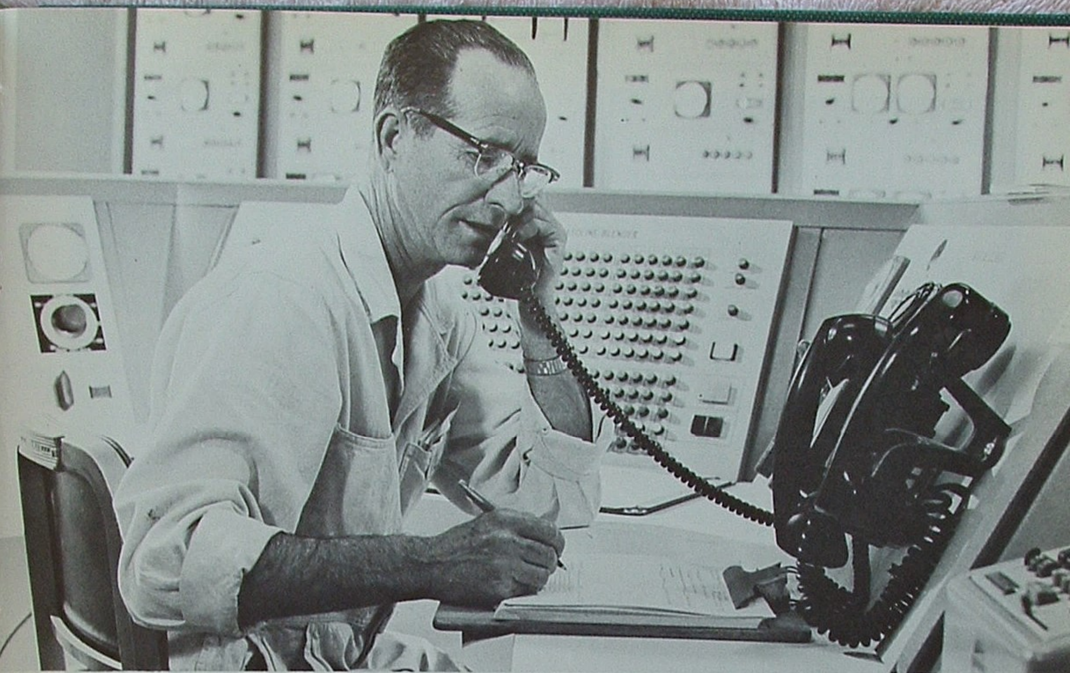
Careful and precise blending of gasoline stocks is the key to top notch performance in your automobile. Here Harold O. Miller sits at the master console of an automated gasoline blending unit at Los Angeles Refinery.
