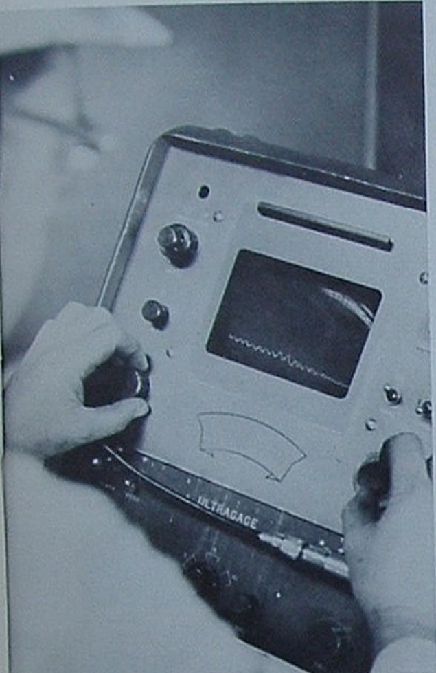
Oscilloscope used to spot corrosion in our refineries.
