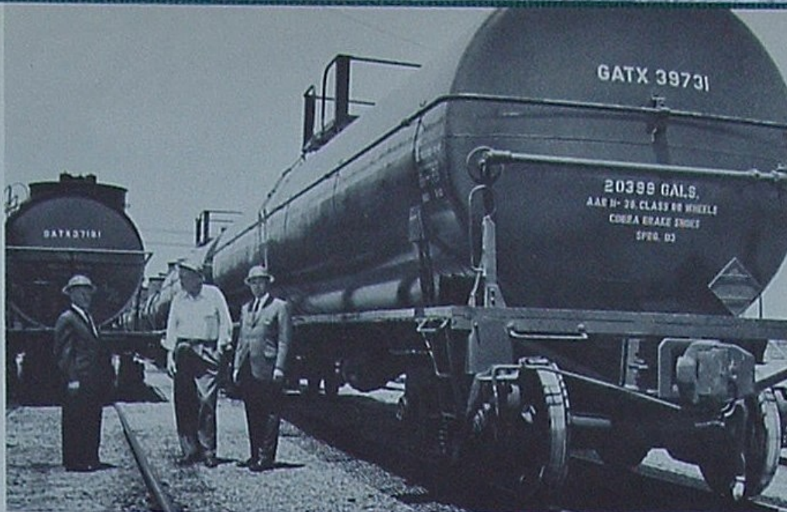
As the supertanker superseded the tanker, so does the super tank car appear to be superseding the regular railway tank car. Here is one of five new 20,000 gallon super tank cars recently delivered to Union's 300-car rail tanker fleet. The five, with twice the capacity of older tank cars, deliver asphalt from Los Angeles Refinery to Arizona. Giving the scene the once over are Ralph Young, tank car analyst at Union Oil Center; Bill Davis, shipping foreman at Los Angeles Refinery; and John P. Ennis, traffic supervisor at UOC.
