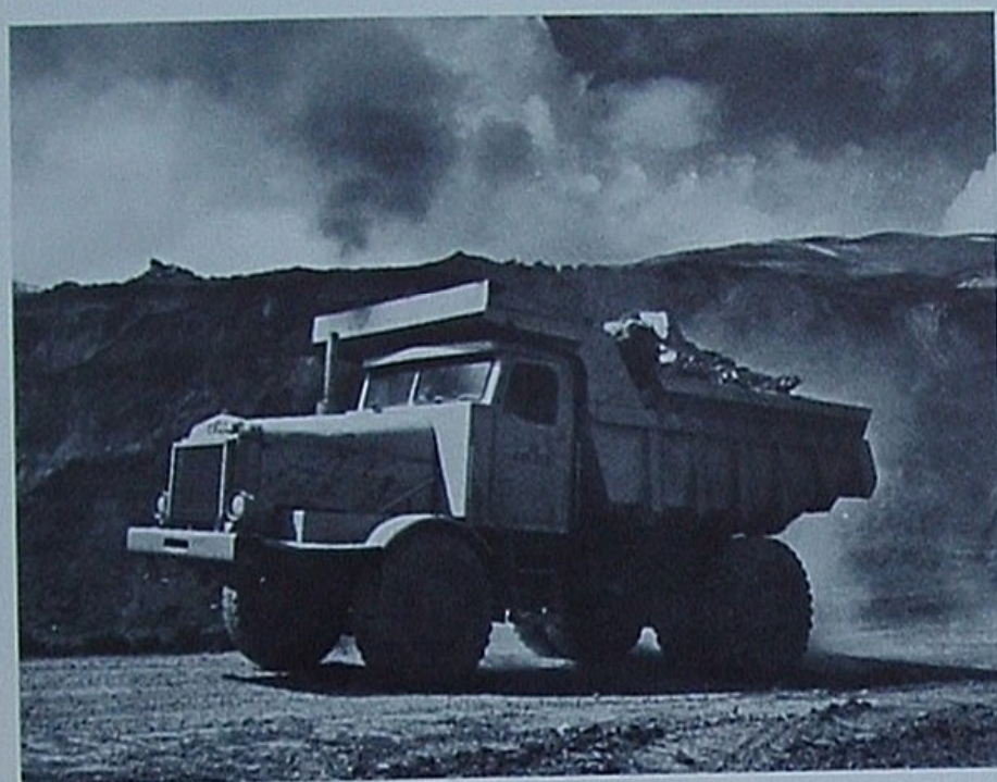
Rugged Euclid truck (left) hauls the ore and waste rock from three open-pit locations. Ore assaying a sufficiently high gold content is trucked to the mill (below) for crushing, processing and melting into bars of gold.
