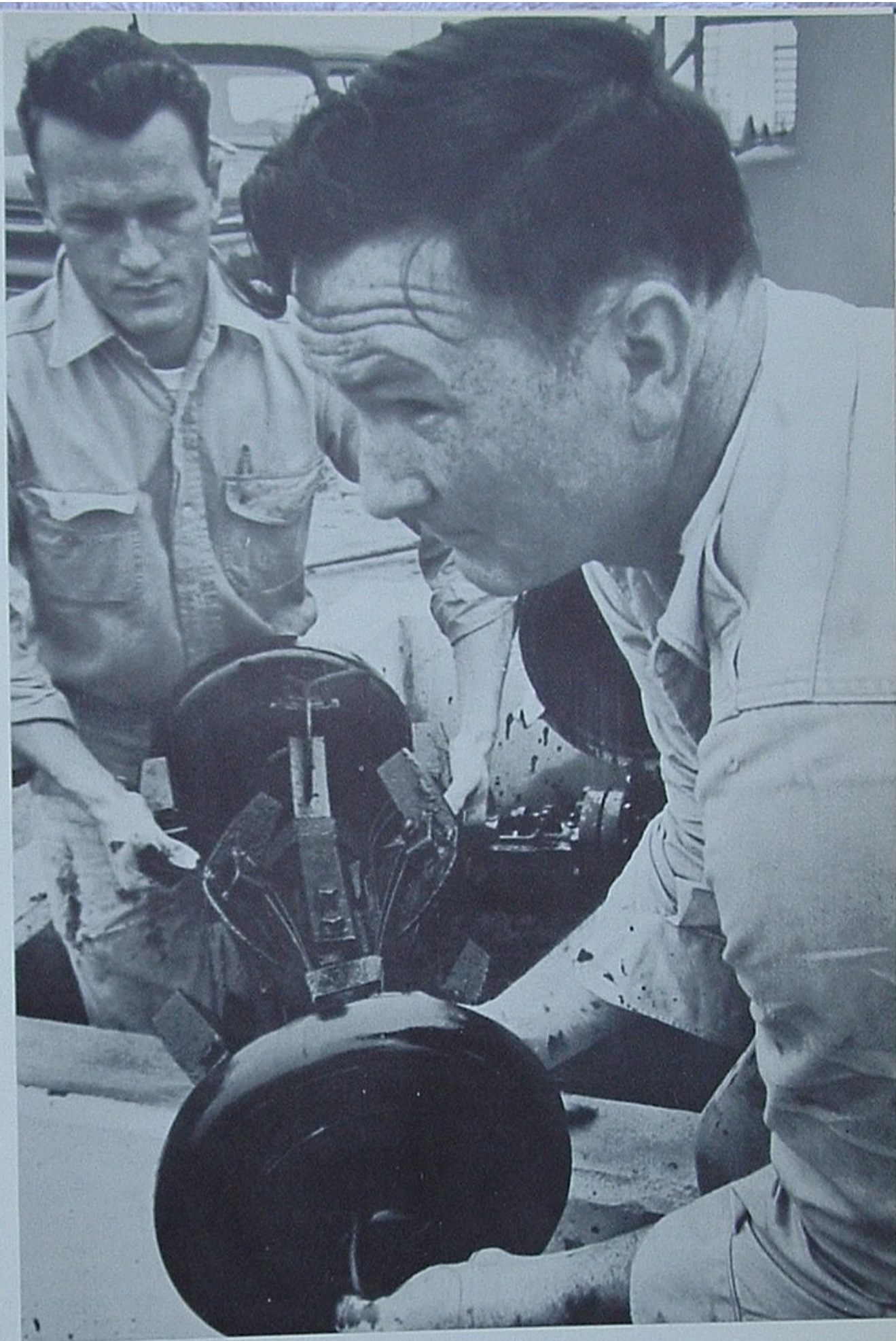
Gary Meyer and Joe Csiszer pull a greased "pig" from a pipeline.
