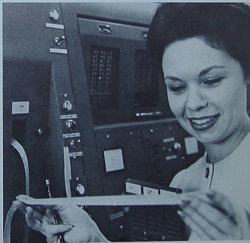
Messages carried by the Company's own teletype lines come into Union Oil Center punched in the tape. Terry feeds the tape into a printer which types copies that wind up on someone's desk—or relays the message to other points.
